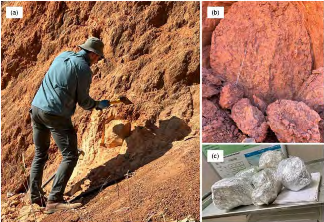
Figure 5-3 (a) Retrieving an undisturbed sample; (b) example of an undisturbed sample; (c) wrapped and stored undisturbed samples (photographed by Dippenaar 2024).
