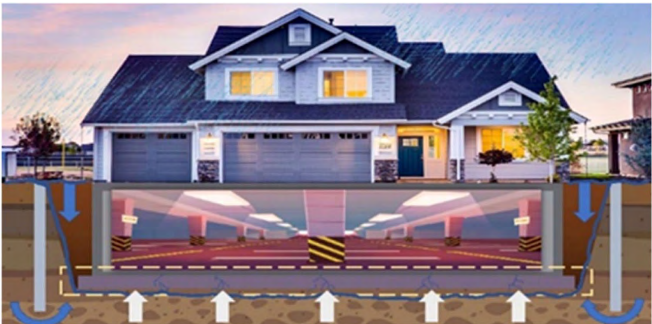
Figure 4-8 Groundwater level rise around the basement leads to leakage (Yue et al. 2024).
