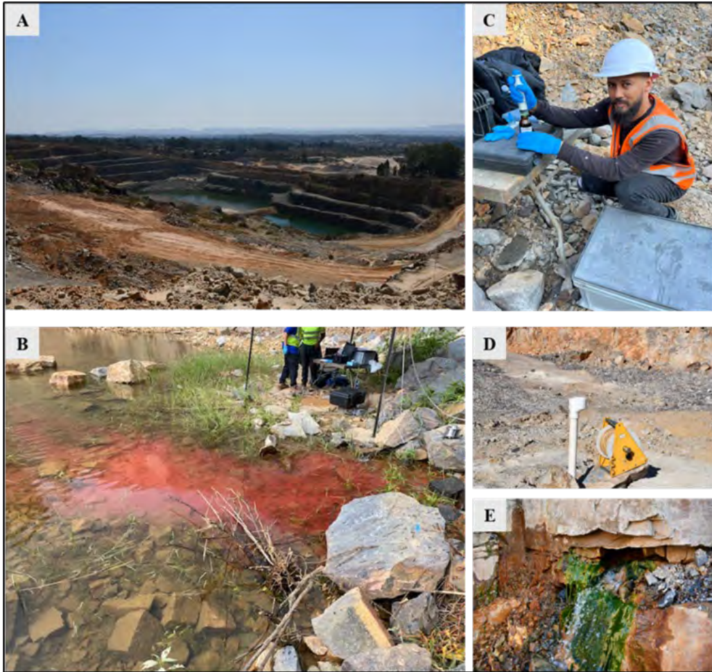
Figure 4-15 Experimental set-up for tracer monitoring using the GGUN-FL30 fluorometer (photographs by van Wyk, 2023).
