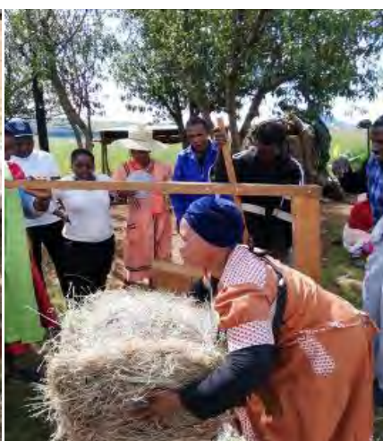
Hand operated baler, with a bale of veld grass made with this baler
