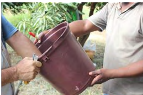
A small hole is made at the bottom of the 20 L bucket to connect the elbow connector and the down pipe
