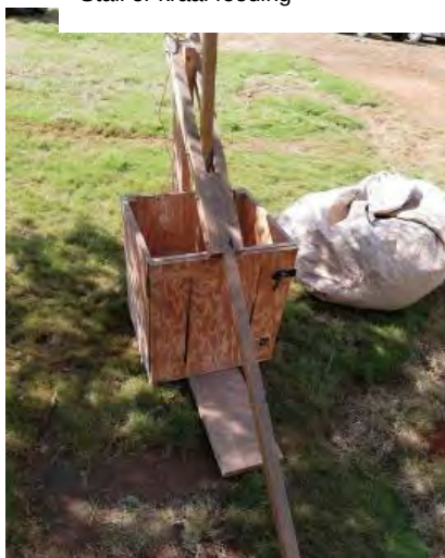
Hand operated baler, with a bale of veld grass made with this baler
