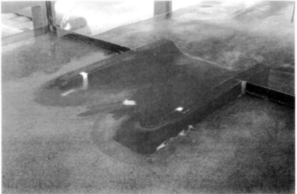
**FIGURE 6.12 - Flume (Layout 2) almost completely cleared after 3 minutes**
