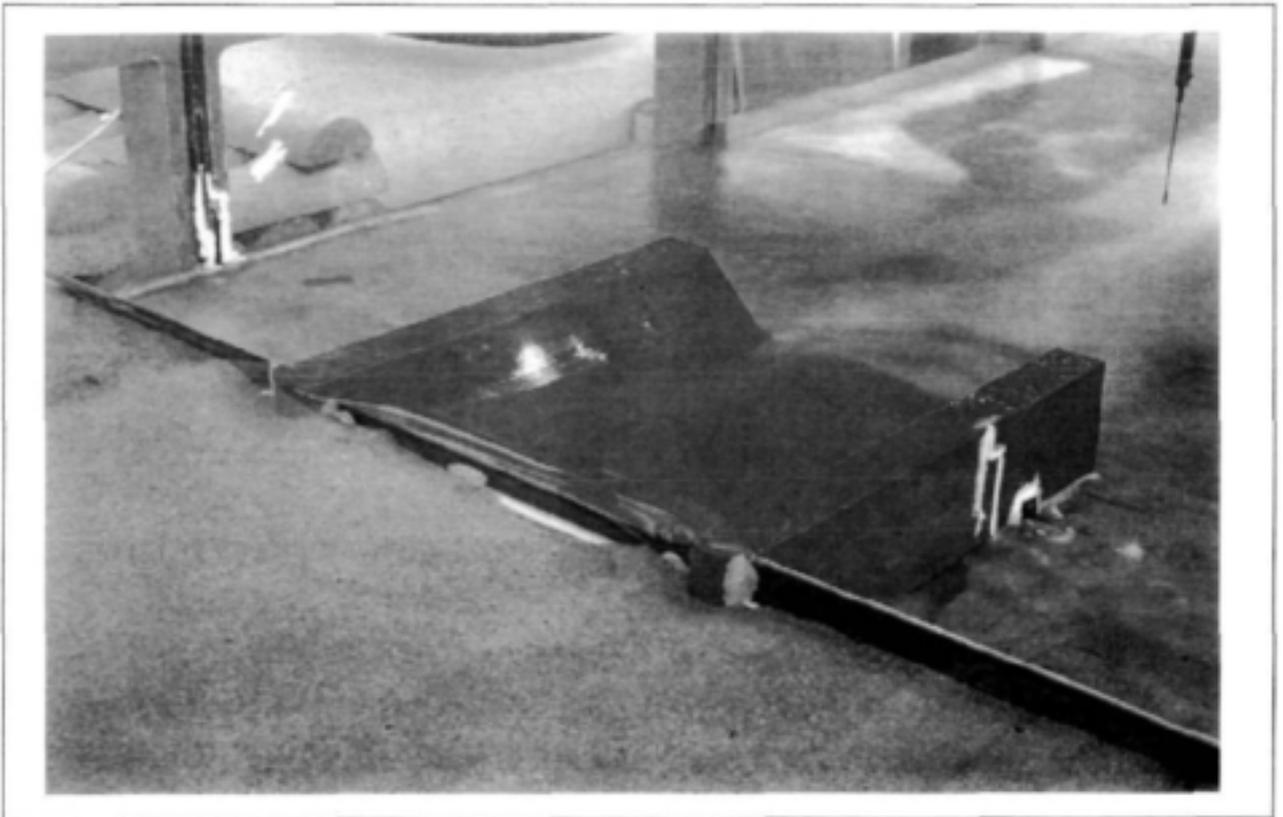
**FIGURE 6.6 - Flume with high step in mouth**
