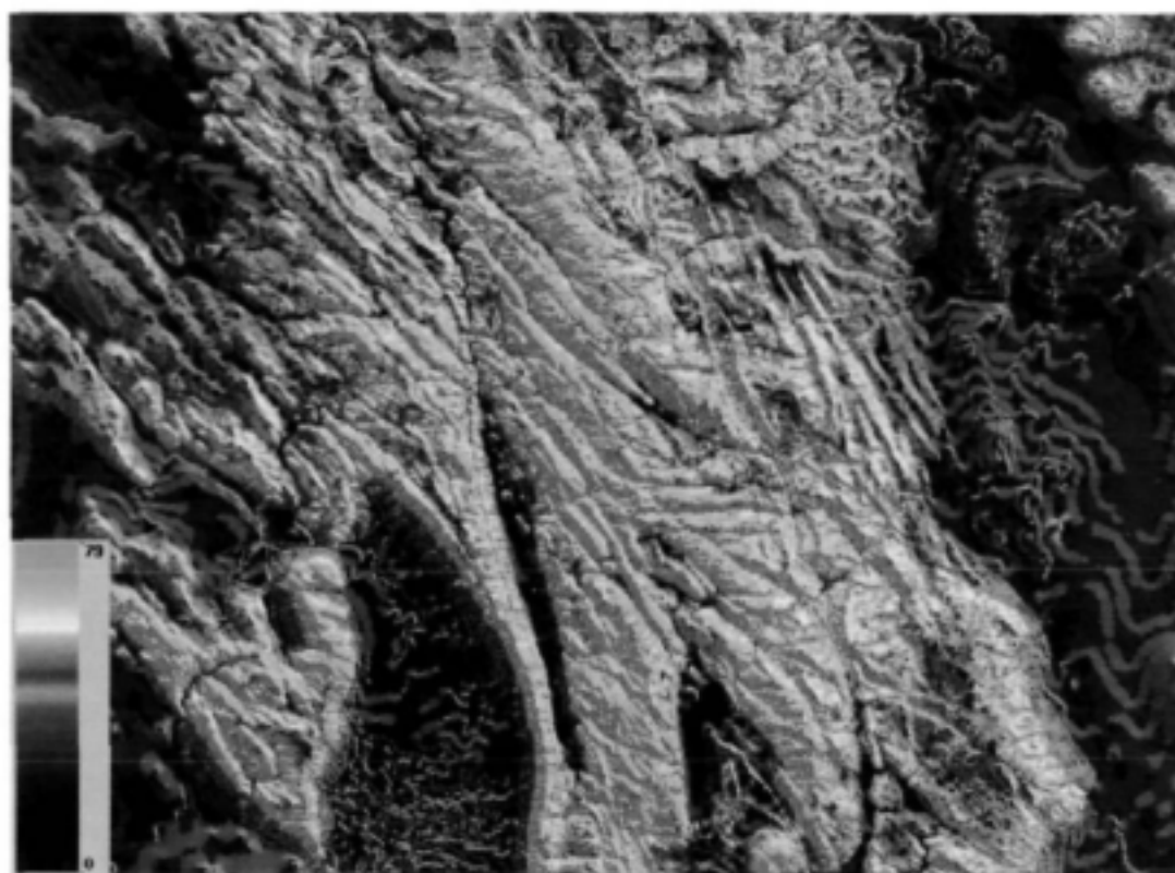
Figure 5 Slope model for the Citrusdal area, created from a Digital Elevation Model. Each 30 x30 m image cell stores a local slope value, useful as input into runoff - infiltration modelling algorithms
