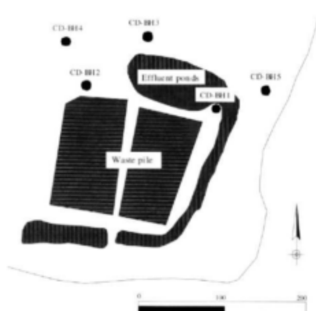
Figure 2 Position of boreholes at Ceres waste disposal site
