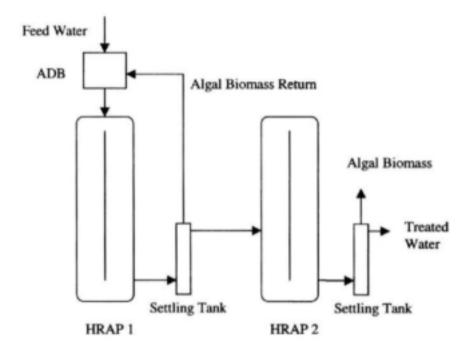
Figure 8.3. Configuration of the Independent-High Rate Algal Pond (I-HRAP) for Nitrogen and Phosphate removal. Influent water and algal biomass, recycled as the carbon source, passes through the Algal Denitrification Bioractor (ADB). Phosphate removal occurs in both HRAP 1 and 2.
