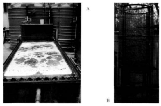
Figure 7.20 The Floating Sulphur Biofilm Reactor (A) and the Silicone Tubular Sulphur Bioreactor (B).
