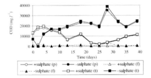
Figure 7.6. The concentration of COD within the bed of the first of the multiple-stage bench-scale reactors fed primary sewage sludge. The total (t), particulate (p) and filtered (f) COD are compared for the sulphate reducing (+ sulphate) and non-sulphate reducing (- sulphate) bioreactor systems.
