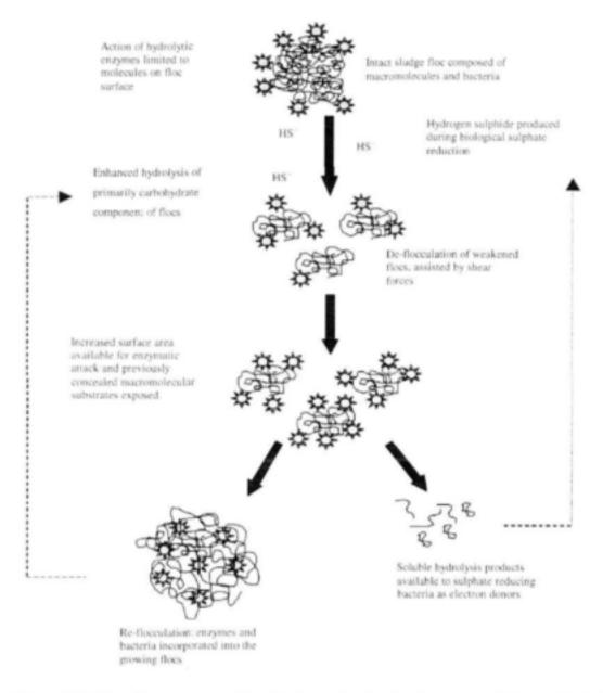
Figure 7.10. Flow diagram summarising the factors involved in the process of enhanced hydrolysis of primary sewage sludge under sulphate reducing conditions.
