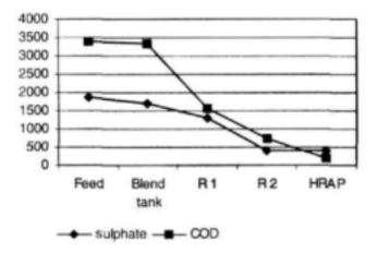
Figure 7.13. Sulphate reduction and COD consumption performance across the various unit operations comprising the Rhodes BioSURE Process<sup>8</sup>. The values represent a period of steady state performance averaged for 1 month process operation.
