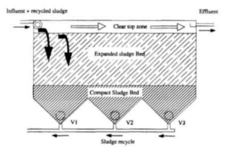
Figure 7.14. The Recycling Sludge Bed Reactor showing the segregation of settled sludge, the recycle of the sludge bed to blend with the incoming flow, and the supernatant liquid carrying the solubilised product to the second stage in the BioSURE Process<sup>\*\*</sup>.
