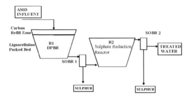
Figure 7.22. The two stage system for Passive Treatment of sulphate-saline mine wastewaters including the Degrading Packed Bed Reactor (DBPR) and its carbon recharge zone, the Sulphate Reduction Reactor unit, and the Sulphide Oxidising Bioreactor (SOBR). Treated water and sulphur are produced as final products.
