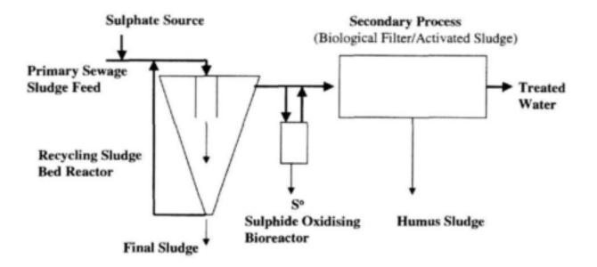
Figure 7.16. Application of the BioSURE Process<sup>®</sup> in the solubilisation of primary sewage sludge. The solubilised fraction passes from the Recycling Sludge Bed Reactor to a secondary process where organics are converted to a humus sludge, and treated water is produced. A final sludge containing metals, cysts and ova is recovered in a small volume from the Recycling Sludge Bed Reactor. Reduced sulphate may be recovered as S<sup>®</sup> in a Sulphide Oxidising Bioreactor.
