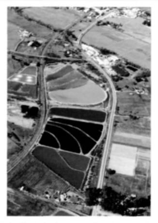
Figure 4.1. The Waste Stabilisation Pond evaporative disposal system treating tannery wastewaters at the Mossop-Western Leathers Co. Wellington. This unit was used as a model in the investigation of ponding systems reported in this study.
