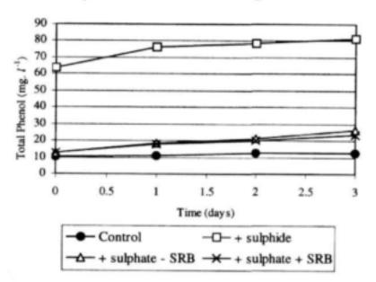
Figure 7.9. The effect of sulphide and sulphate reduction on the concentration of total soluble phenol in primary sewage sludge when digested anaerobically. The +sulphide value represents an elevation from 10.2 to 63.5 mg.L<sup>-1</sup> phenol within a period of a few minutes.
