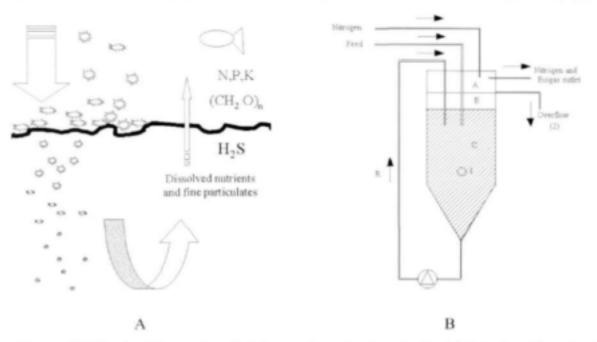
Figure 7.4. The breakdown of particulate organic matter in natural sulphidogenic settlement and sedimenting processes (A) was simulated in a 1L prototype study (B) of the Recycling Sludge Bed Reactor (RSBR). The degrading sludge is returned via line R to blend with the incoming feed.
