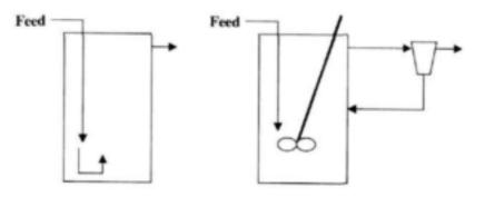
Figure 7.3. Comparison of two sulphate reducing reactor configurations. The bottom-fed upflow reactor (A) and the stirred tank reactor (B) with sludge recycle.
