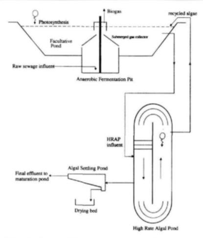
Figure 8.1. Schematic diagram of the IAPS demonstration and research plant constructed at the Environmental Biotechnology Field Station in Grahamstown as a component of the IAPS research facility.
