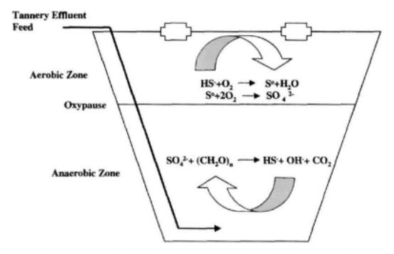
Figure 5.5. The primary facultative pond of the LAPS system treating tannery wastewaters after reconfiguration, using surface aerators in establishing a stable oxypause, and relocating feed inlet to the bottom of the pond.
