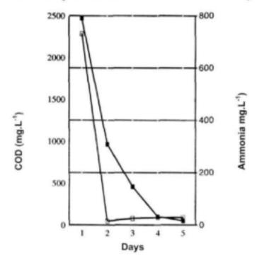
Figure. 5.2. COD and ammonia removal in a *Spirulina* photobioreactor showing a typical 5-day batch fed sequence with a tannery effluent loading rate equivalent to 5% reactor volume.day<sup>-1</sup>. (Closed square=COD; open square=ammonia).
