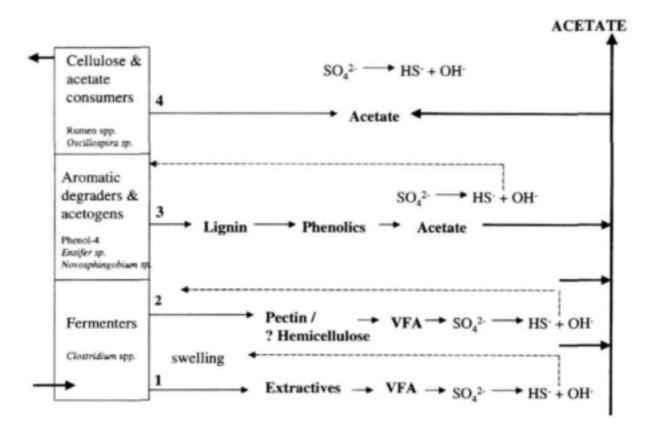
Figure 7.21. A descriptive model of events occurring in the mobilisation of lignocellulose as carbon and electron donor source in experimental wood chip packed columns. A molecular microbial ecology study of the system provides an explanation of processes occurring at each level.
