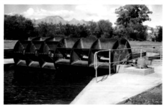
Figure 3. Paddle wheel of the industrial-scale 2500 m<sup>2</sup> Spirulina-HRAP constructed in Wellington, South Africa, for the treatment of tannery wastewaters.
