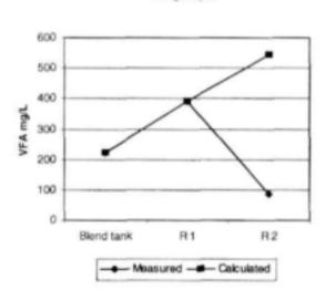
Figure 7.15. Volatile fatty acid production from primary sewage sludge in the BioSURE<sup>®</sup> pilot plant. Actual values measured across the system are compared with calculated values for total VFA production, based on COD consumed (as acetate) in sulphate reduction.
