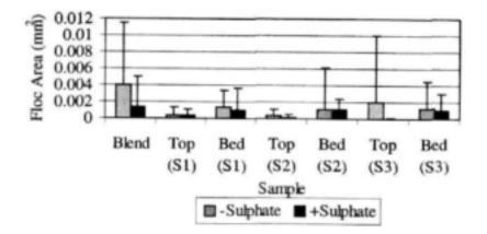
Figure 7.7. Mean area of sludge flocs within the feed and three stages of the sulphidogenic (+ sulphate) and non-sulphidogenic (- sulphate) multiple-stage bench-scale bioreactors. Bars indicate standard deviations and the primary sludge feed values for both systems were equivalent to the –sulphate blend value.
