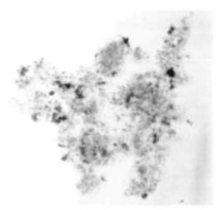
Figure 7.8. Floc morphology showing the dense particulate matter embedded within extracellular polymeric materials (light microscope 40x magnification).
