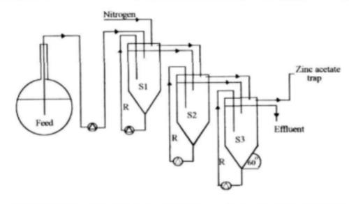
Figure 7.5. The multi-stage Recycling Sludge Bed Reactor used to investigate the solubilisation of primary sewage sludge and its utilisation as an electron donor source in sulphate reduction activity.
