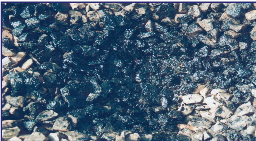
Figure 2.2(b): Exposure of Iron Sulphide Solids Blocking the Filter Media
