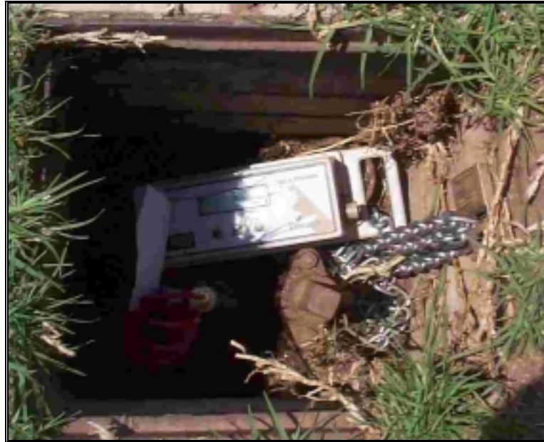
Figure 2.2 : Pressure logger installation on a fire hydrant
