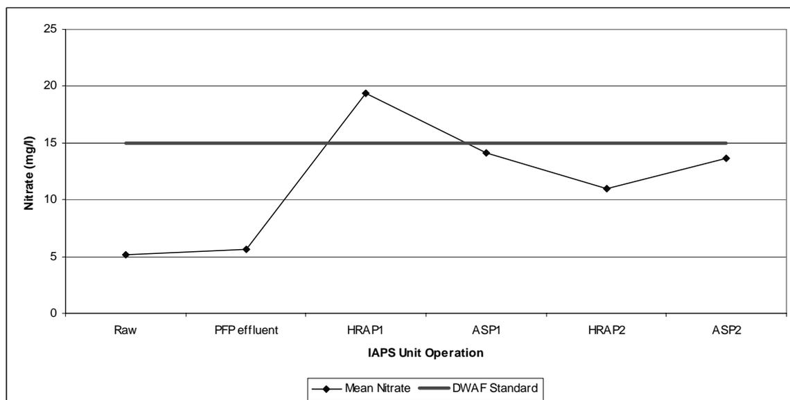
**Figure 5:** Average values for nitrate cycling through the IAPS, monitored over the period 1997-2004. HRAP2 and ASP2 were only brought online as the I-HRAP operation in July 2003. . PFP = Primary Facultative Pond, HRAP = High Rate Algal Pond, ASP = Algal Settling Pond.
