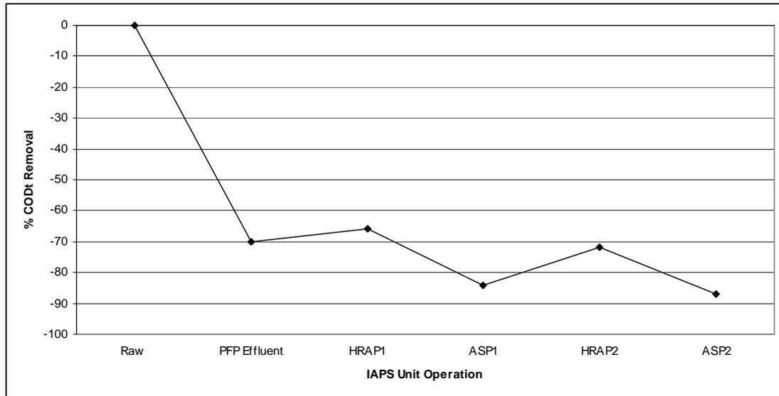
**Figure 10.1:** Total chemical oxygen demand removal through the integrated algal ponding system. The results depicted for the raw water, PFP effluent, HRAP1 and ASP1 reflect averages for HRAP treatment for the entire period from July 1996 to October 2004. HRAP2 and ASP2 were only brought online as the I-HRAP operation in July 2003.
