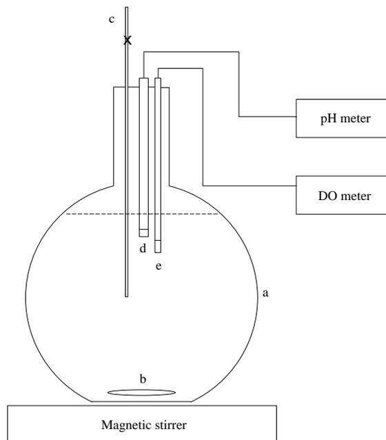
**Figure 9.1:** Experimental apparatus used for batch denitrification experiments. (a) Foil covered glass flask (b) magnetic follower (c) sampling port (d) pH-electrode (e) DO-electrode.
