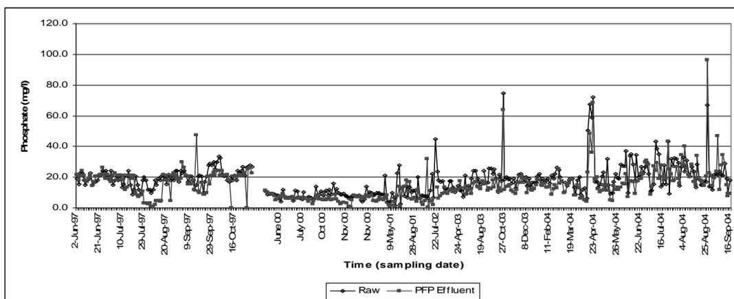
**Figure 4.9:** Comparison of phosphorous as  $\text{mg}\cdot\ell^{-1} \text{PO}_4^{3-}$  in the sewage feed (raw) and primary facultative pond effluent during the period June 1997 to September 2004.
