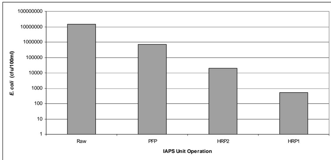
**Figure 10.5:** *E. coli* counts through the IAPS and I-HRAP sequence. This figure illustrates all data from the 2003-2004 monitoring period, i.e. including results from operation with sub-optimal hydraulic retention times.
