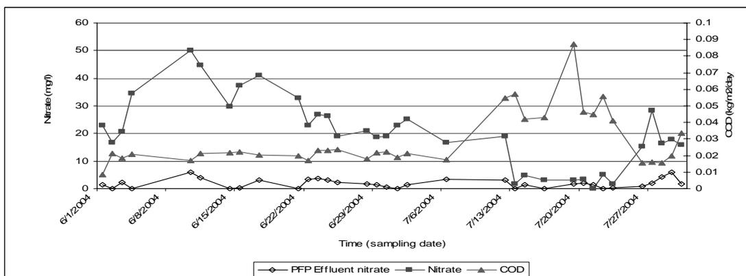
**Figure 5.8:** Nitrate in the high rate algal pond plotted against chemical oxygen demand load to the high rate algal pond, and illustrating a drop in nitrate levels at high organic loading.
