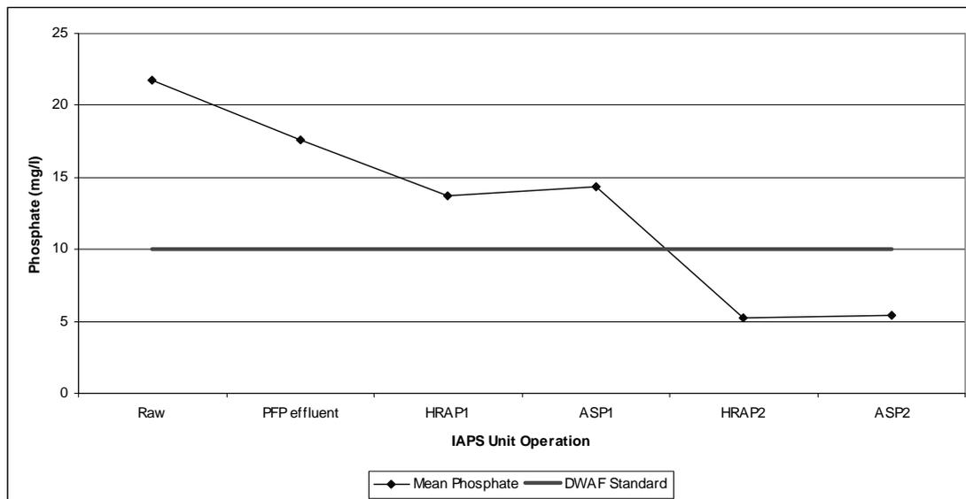
**Figure 10.4:** Average results for phosphate removal in the IAPS, monitored over the period 1997-2004. I-HRAP (HRAP2 and ASP2) averages for 2003-2004.
