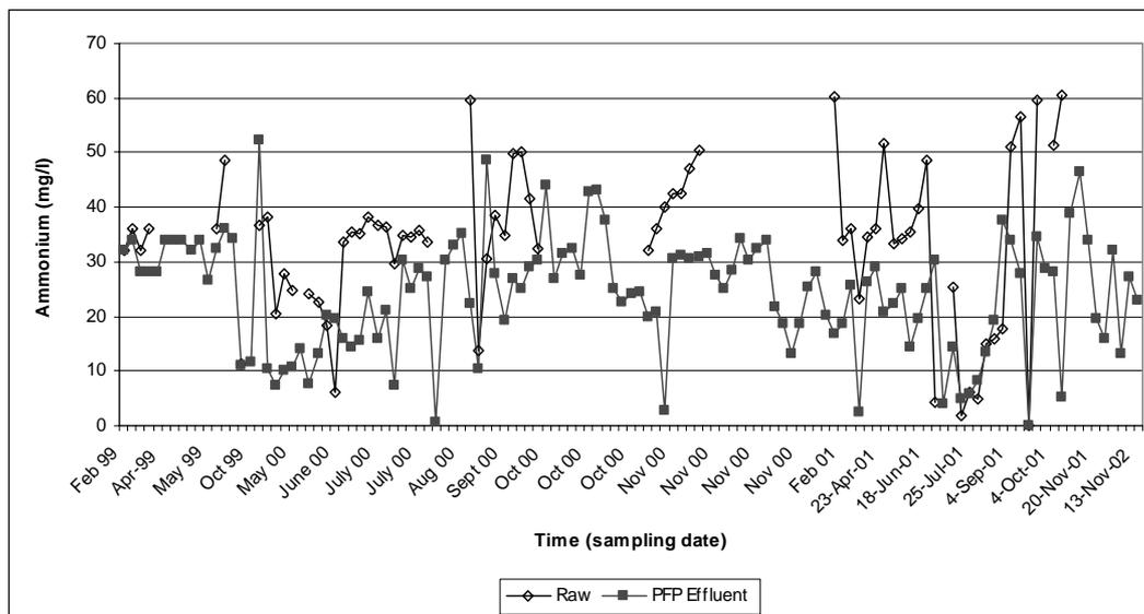
**Figure 4.7:** Comparison of nitrogen as  $\text{mg}\cdot\ell^{-1} \text{NH}_4^+$  in the sewage feed (raw) and primary facultative pond effluent during the period February 1999 to November 2002.
