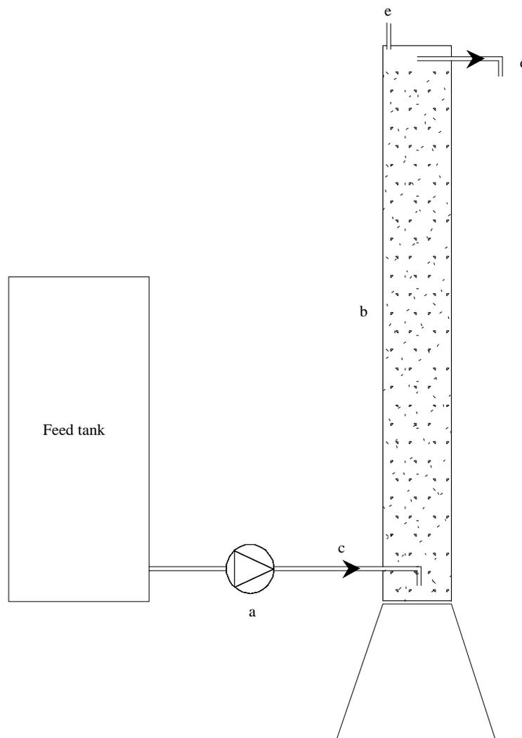
**Figure 9.2.** Upflow anoxic column with settled algal biomass. (a) Peristaltic pump (b) covered cylindrical glass column (c) influent (d) overflow (e) gas vent.
