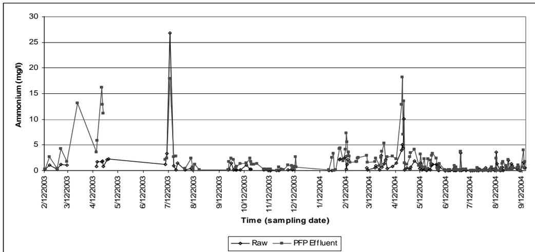
**Figure 4.8:** Comparison of nitrogen as  $\text{mg}\cdot\ell^{-1} \text{NH}_4^+$  in the sewage feed (raw) and primary facultative pond effluent during the period February 2003 to September 2004.
