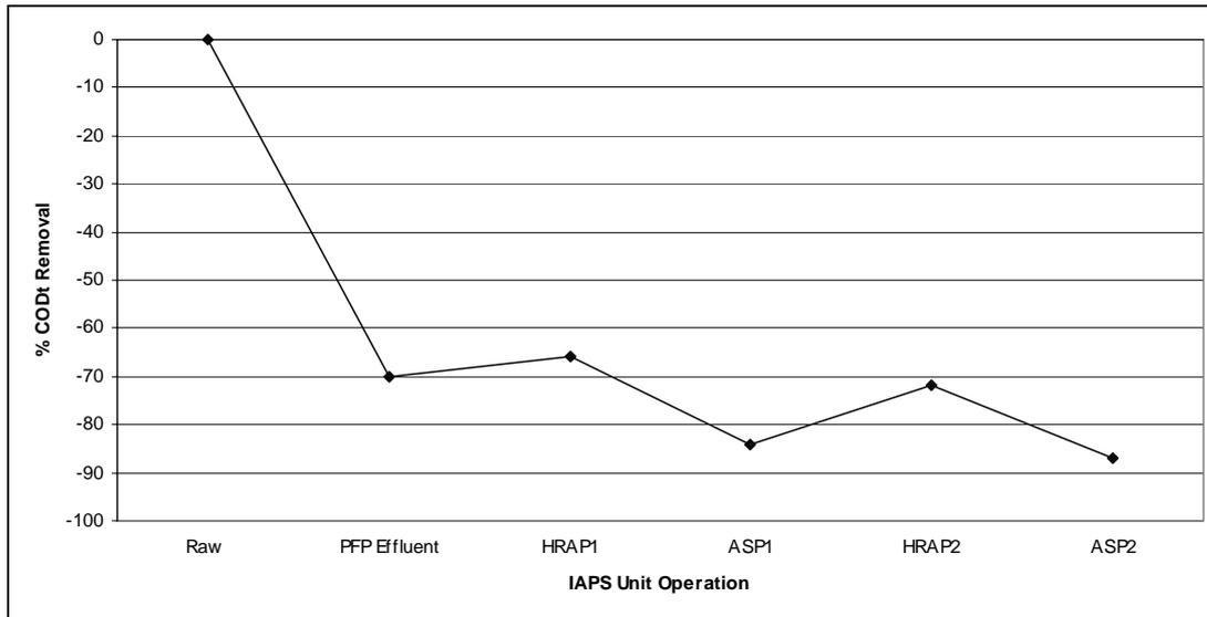
**Figure 3:** Total chemical oxygen demand removal through the integrated algal ponding system. The results depicted for the raw water, PFP effluent, HRAP1 and ASP1 reflect averages for HRAP treatment for the entire period from July 1996 to October 2004. HRAP2 and ASP2 were only brought online as the I-HRAP operation in July 2003. PFP = Primary Facultative Pond, HRAP = High Rate Algal Pond, ASP = Algal Settling Pond.
