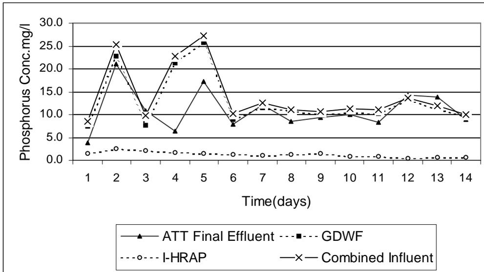
**Figure 9.9:** Phosphate release in the algal denitrification packed column reactor showing influent phosphate and algal load drawn from the I-HRAP, and set at a hydraulic retention time of 48 hours.
