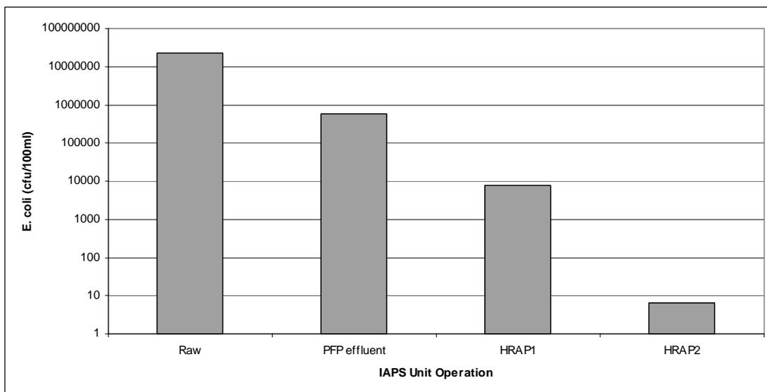
**Figure 8:** *E. coli* counts through the IAPS and I-HRAP sequence, illustrating results only from operation under optimal hydraulic retention times, both during 2003 and 2004. . PFP = Primary Facultative Pond, HRAP = High Rate Algal Pond.
