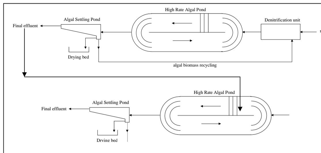
**Figure 9.11:** I-HRAP tertiary treatment process conceptualisation including denitrification of the influent stream with the use of algal biomass as carbon source.
