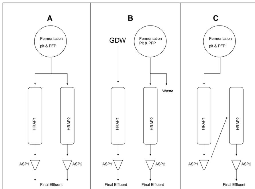
**Figure 2:** Development of the Independent High Rate Algal Pond (I-HRAP) system and showing the various configurations of the HRAP evaluated in this study. PFP = Primary Facultative Pond, ASP = Algal Settling Pond, GDW = Grahamstown Disposal Works.
