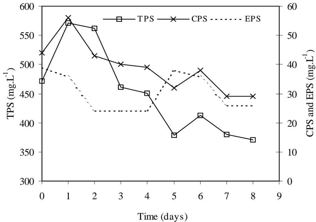
**Figure 9.3:** Batch denitrification using algal biomass as the carbon source and showing (A) repeated replenishment of nitrate against COD consumption and (B) polysaccharide release and utilisation.
