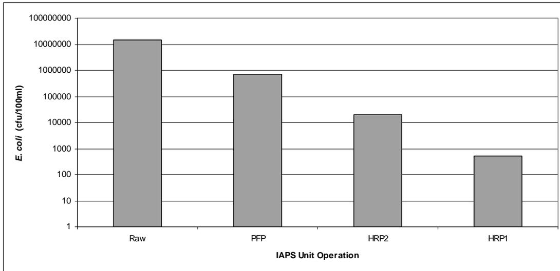
**Figure 7:** *E. coli* counts through the IAPS and I-HRAP sequence. This figure illustrates all data from the 2003-2004 monitoring period, i.e. including results from operation with sub-optimal hydraulic retention times. . PFP = Primary Facultative Pond, HRAP = High Rate Algal Pond.
