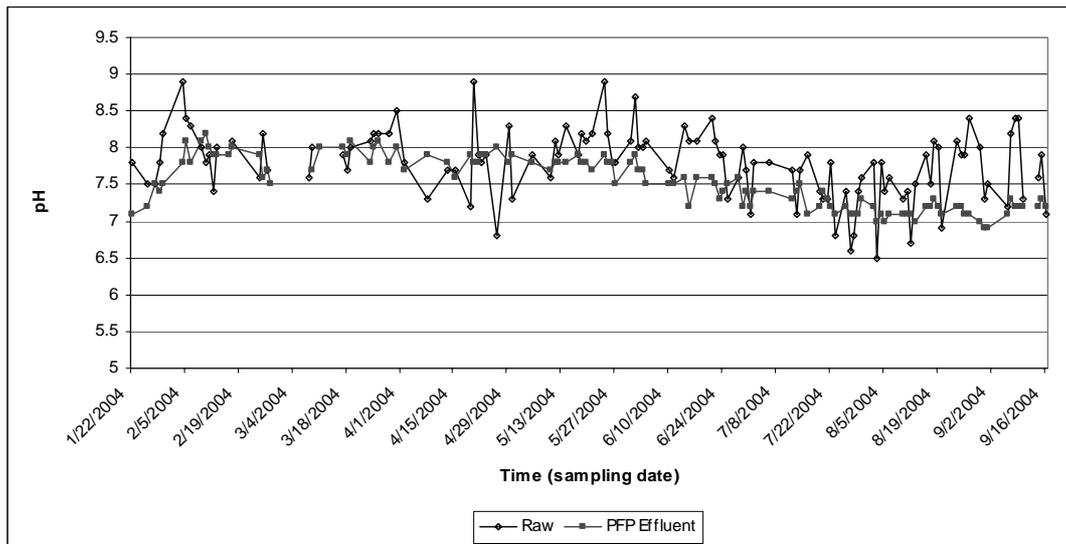
**Figure 4.5:** Comparison of raw and primary facultative pond effluent pH over the sampling period January to September 2004
