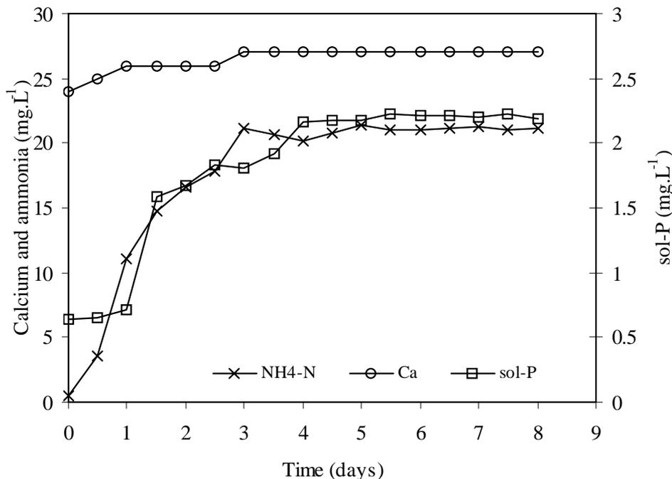
**Figure 9.4:** The release of phosphate and ammonia during denitrification
