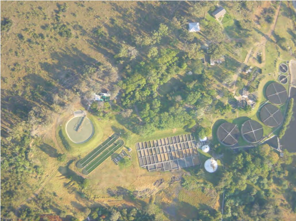
**Figure 3.6:** The primary facultative pond and the integrated algal ponds of the research plant shown at left in relation to components of the Grahamstown Disposal Works shown at right.
