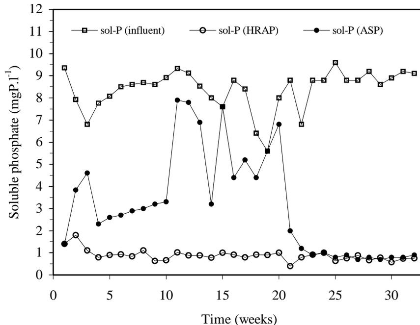
**Figure 7.3.** Release of phosphate from I-ASP during different biomass harvesting procedures.
