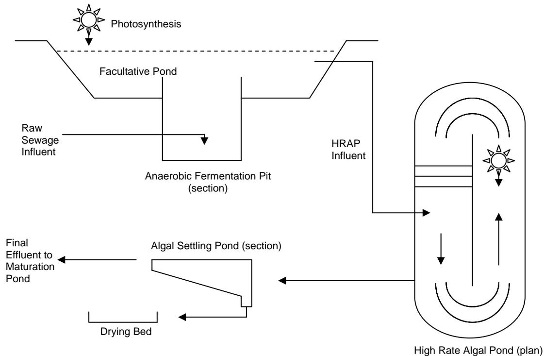
**Figure 2.1** Schematic diagram of the principal unit operations associated with the AIWPS Plant design constructed at the Rhodes University Environmental Biotechnology Experimental Field Station, Grahamstown Disposal Works. After Rose *et al.* (2002c).
