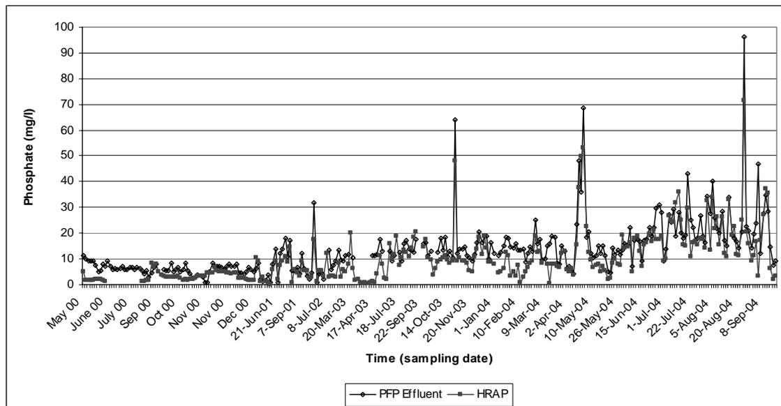
**Figure 5.9:** Phosphate in the primary facultative pond effluent and high rate algal pond during the period May 2000 to September 2004.
