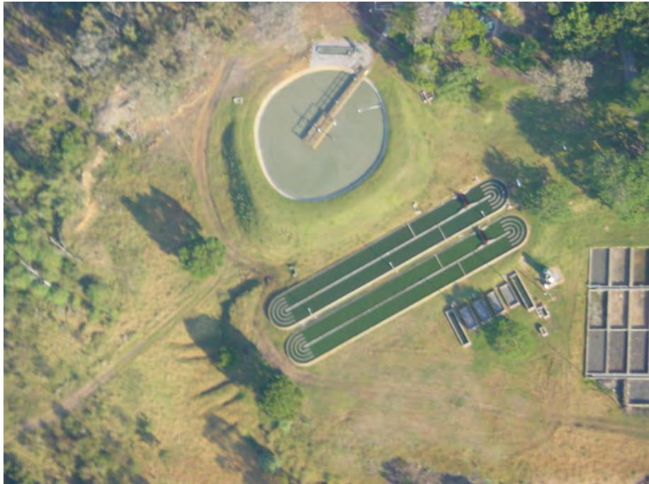
**Figure 3.1:** Aerial photograph of the Integrated Algal Ponding System research plant at the Rhodes University Environmental Biotechnology Experimental Field Station, showing the primary facultative pond (top) and high rate algal ponds, algal settling ponds and drying beds below.
