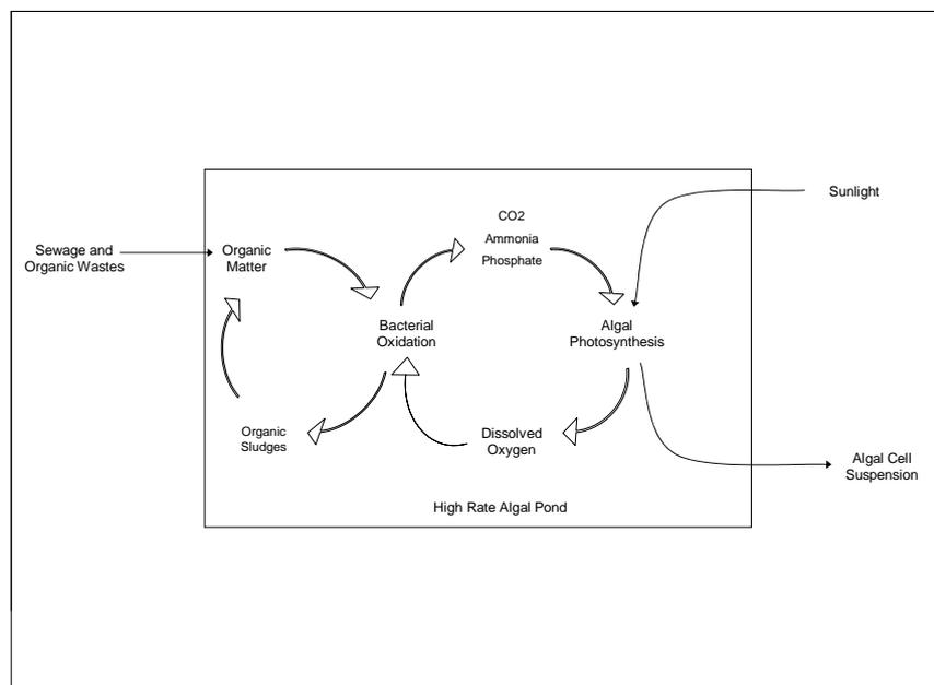
**Figure 5.1:** Cycle for photosynthetic oxygenation of wastewater. After Oswald (1988a)
