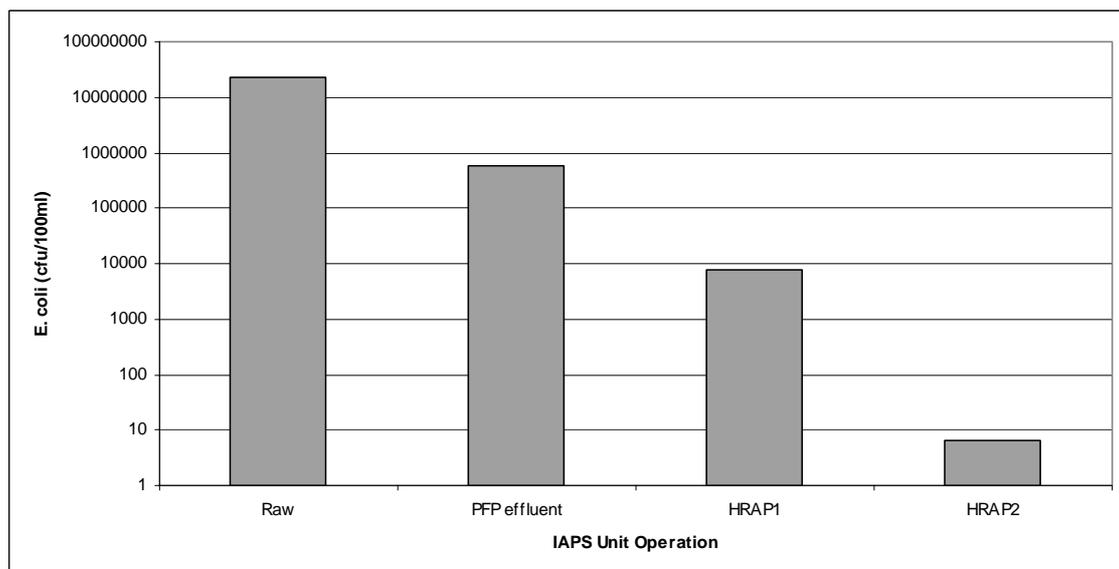
**Figure 10.6:** *E. coli* counts through the IAPS and I-HRAP sequence, illustrating results only from operation under optimal hydraulic retention times, both during 2003 and 2004.
