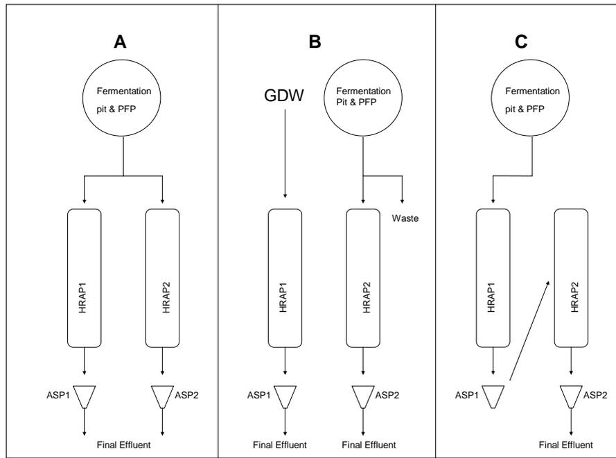
**Figure 3.7:** Various configurations of the HRAP unit operation evaluated in this study.
