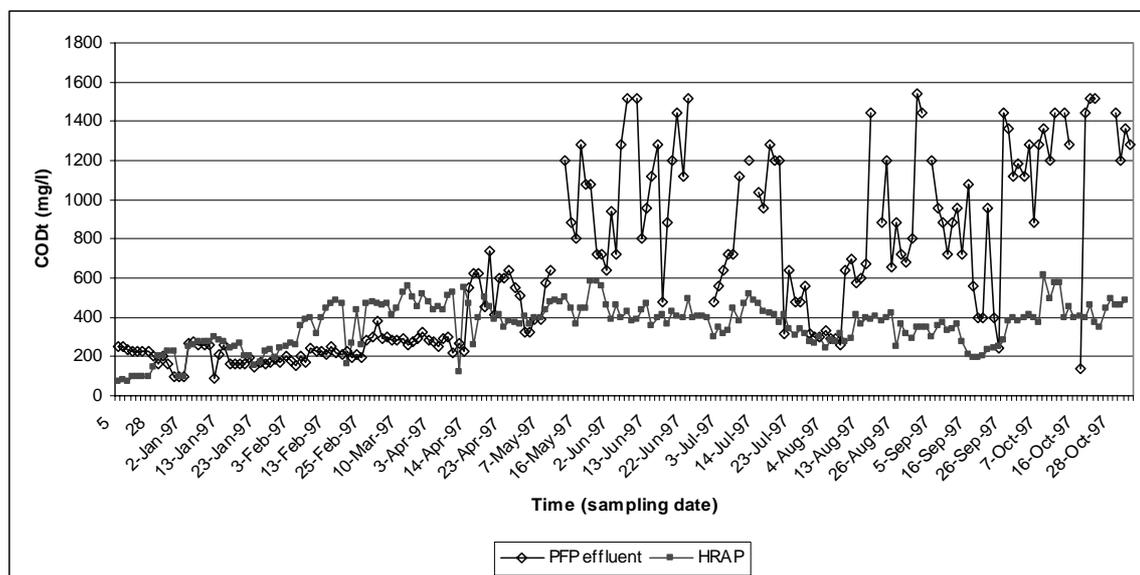
**Figure 5.2:** Unfiltered chemical oxygen demand removal in the first high rate algal pond, during 1997.
