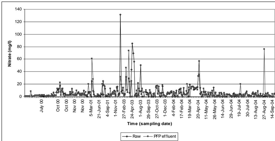
**Figure 4.6:** Comparison of nitrogen as  $\text{mg}\cdot\ell^{-1} \text{NO}_3^-$  in the sewage feed (raw) and primary facultative pond effluent during the period May 2000 to September 2004.
