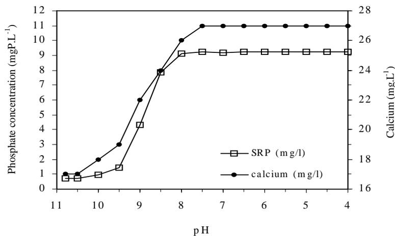
**Figure 7.6.** The release of chemically bound phosphate during the addition of acid, showing the relationship between pH and soluble reactive phosphorus concentration.
