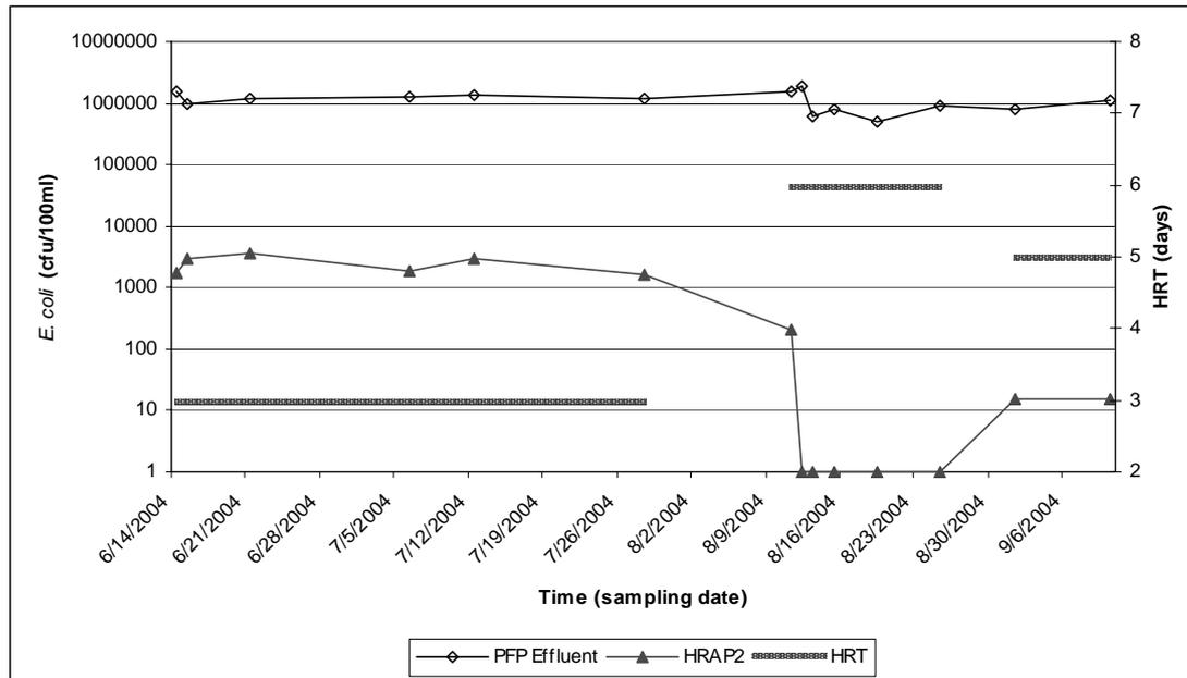
**Figure 6.3:** *E. coli* removal in the IHRAP under winter conditions and with the operation of the system at different hydraulic retention times.
