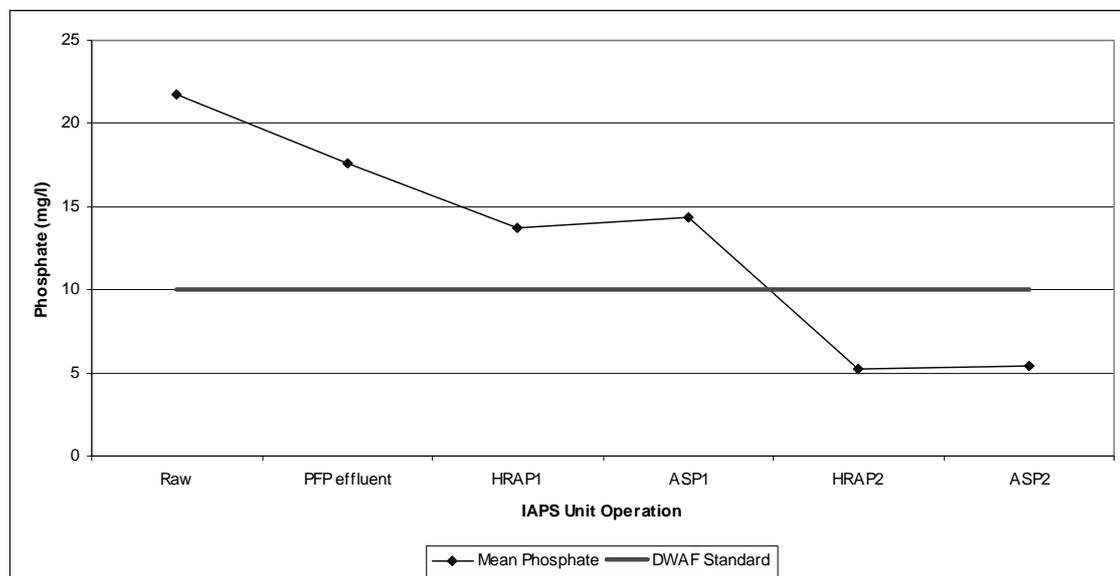
**Figure 6:** Average results for phosphate removal in the IAPS, monitored over the period 1997-2004. HRAP2 and ASP2 were only brought online as the I-HRAP operation in July 2003. . PFP = Primary Facultative Pond, HRAP = High Rate Algal Pond, ASP = Algal Settling Pond.
