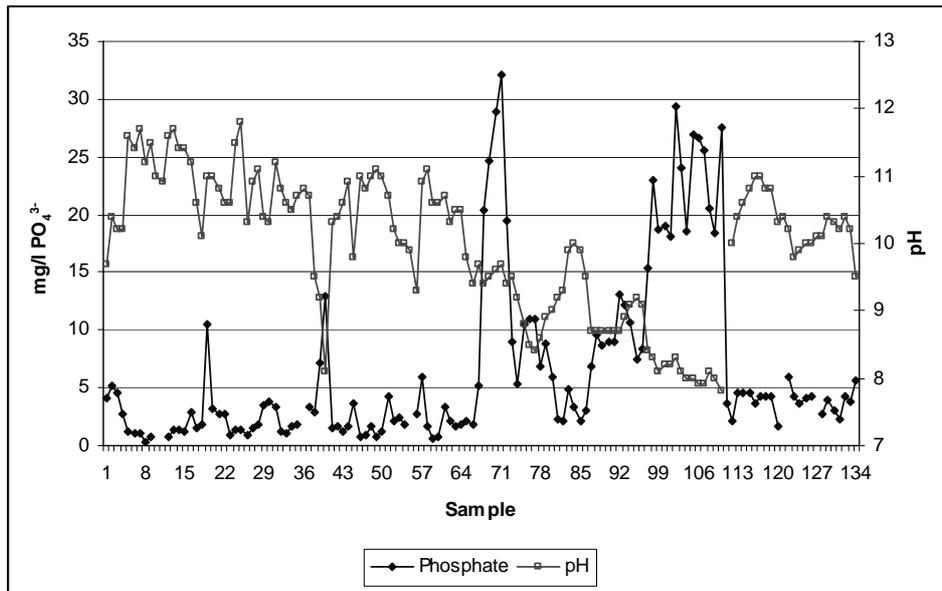
**Figure 7.8:** Phosphate removal showing an inverse relationship with pH.
