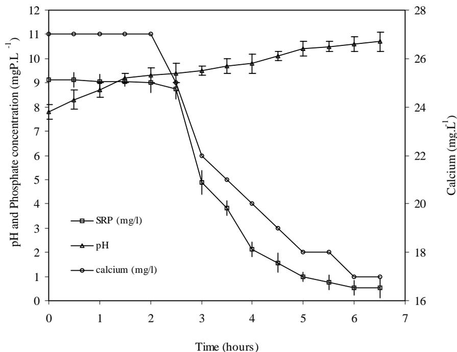
**Figure 7.5.** Precipitation of calcium phosphate minerals from GDW-final in the presence of photosynthesising algae.
