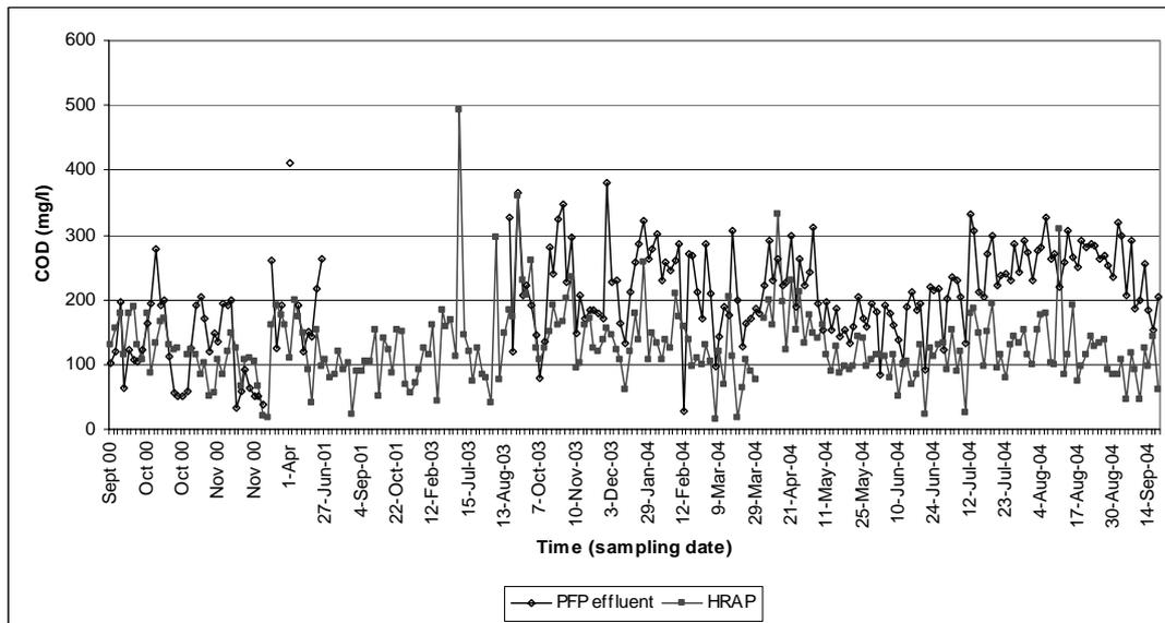
**Figure 5.4:** Soluble chemical oxygen demand removal in the high rate algal pond for the period September 2000 to September 2004.
