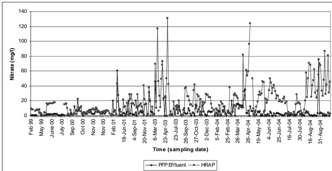
**Figure 5.5:** Nitrate in the primary facultative pond effluent and high rate algal pond for the period February 1999 to August 2004
