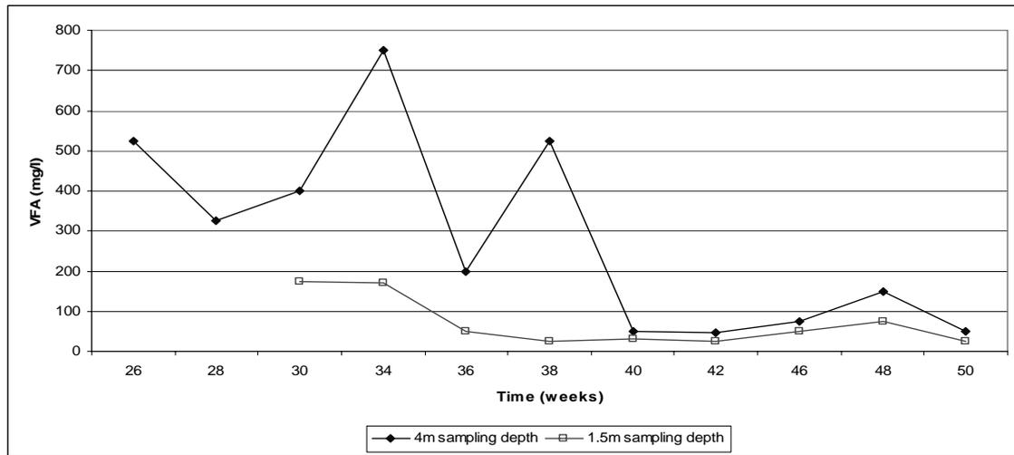
**Figure 4.1:** Stabilisation of volatile fatty acid levels in the fermentation pit, during commissioning and after reseeded with anaerobic sludge from the Grahamstown Disposal Works.
