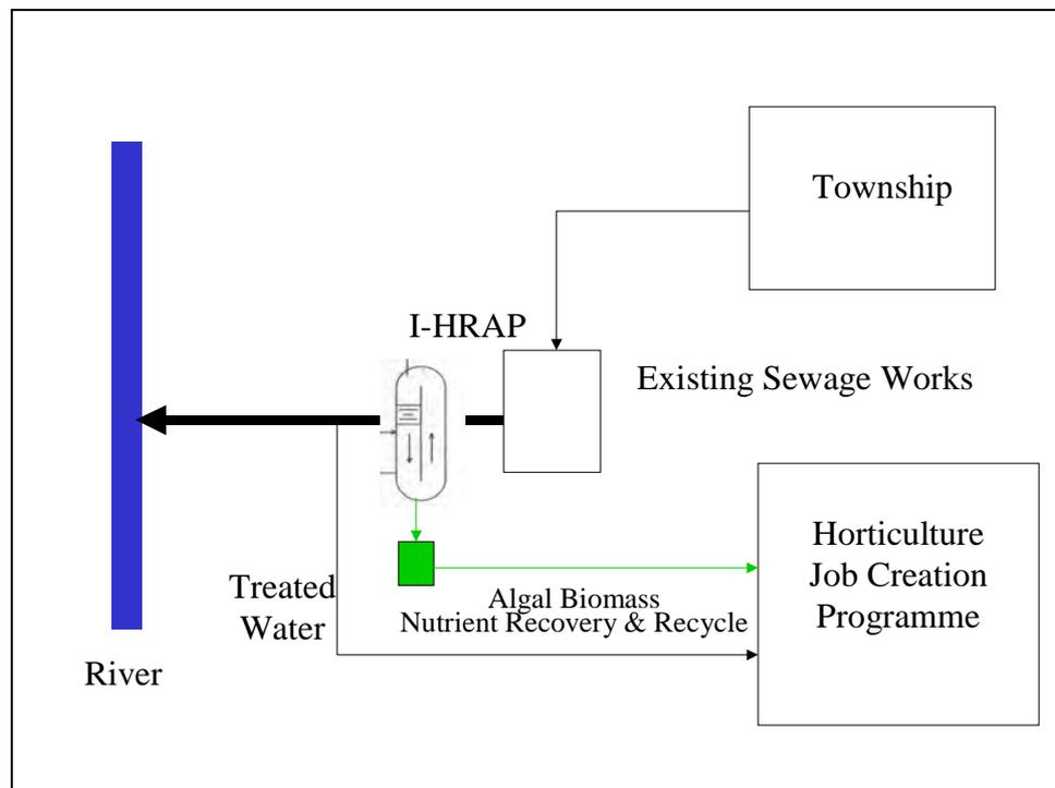
**Figure 11.1:** A schematic outline of the application of the I-HRAP as a retrofit to an existing poorly performing sewage works. Tertiary treatment, including disinfection, would enable the recovery and re-use of the water resource, and algal biomass as fertiliser, in community gardening or urban agriculture job creation projects.
