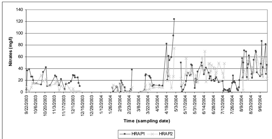
**Figure 8.2:** A 1-year study of nitrate removal in the I-HRAP treating final water from the IAPS plant.
