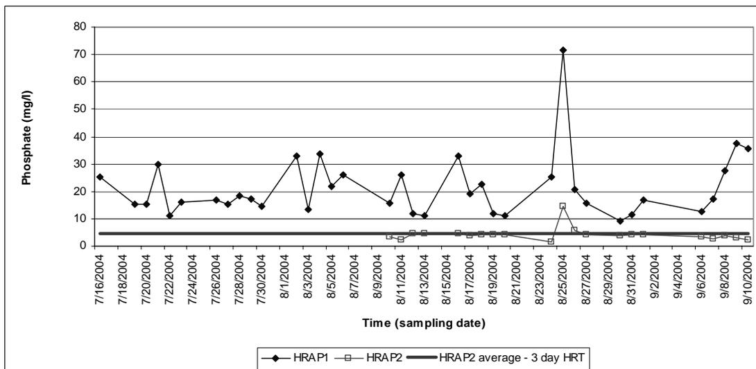
Figure 8.4: Comparison of phosphate removal in the HRAP at a 6 day hydraulic retention time (HRAP1) compared to the I-HRAP following the IAPS configuration (HRAP 2) operated at a 3 day HRT.
