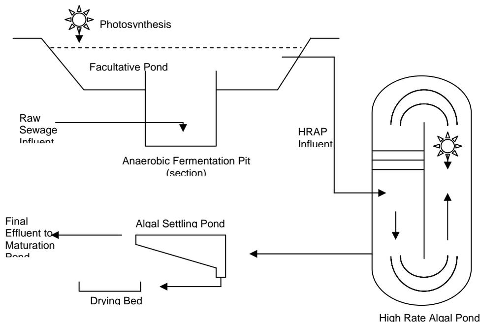
**Figure 1:** Schematic diagram of the principal unit operations of the IAPS Plant constructed at the Rhodes University Environmental Biotechnology Experimental Field Station, Grahamstown Disposal Works. After Rose *et al.* (2002c).
