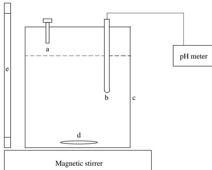
**Figure 7.1:** Culture apparatus used for algal mediated experiments with the following components: (a) small sampling port; (b) pH electrode; (c) 1-litre cylindrical glass vessel; (d) magnetic follower; (e) fluorescent tube x 6.
