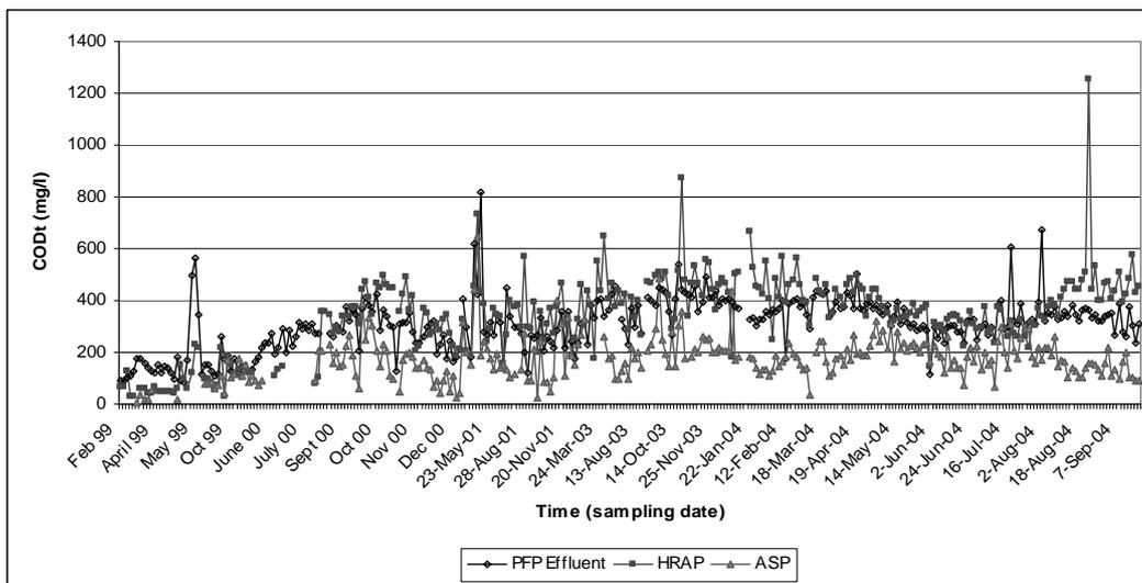
**Figure 5.3:** Unfiltered chemical oxygen demand removal in high rate algal pond 1 and algal settling pond 1 for the period February 1999 to September 2004.
