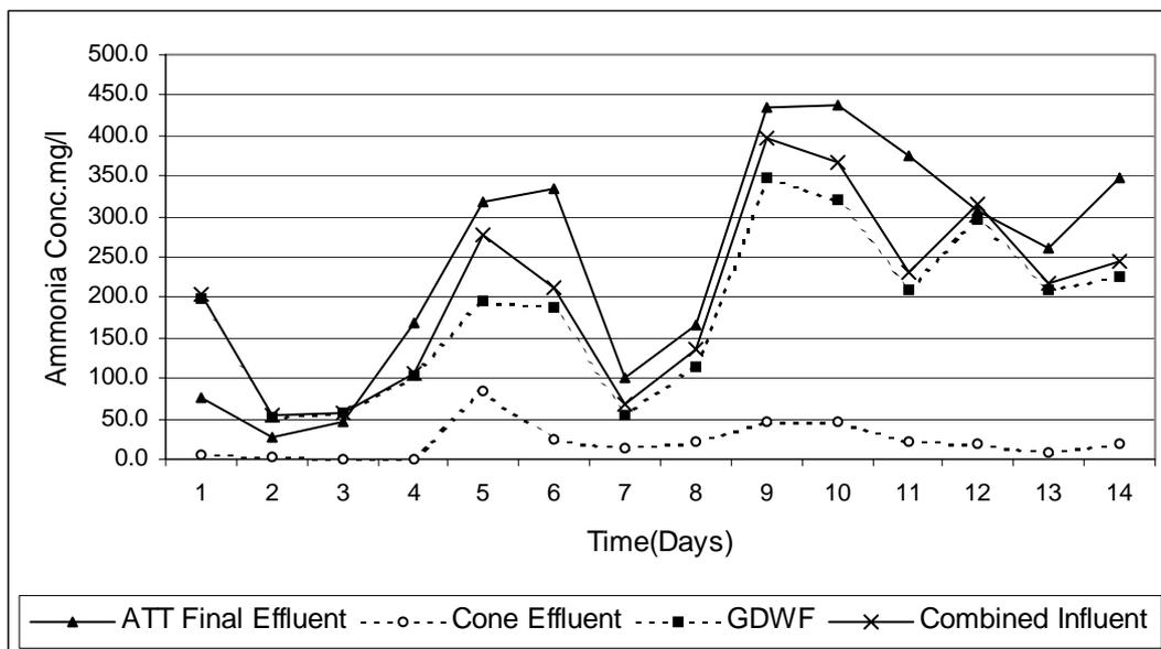
**Figure 9.10:** Ammonia production in the algal denitrification packed column reactor showing influent ammonia and algal load drawn from the I-HRAP, and set at a hydraulic retention time of 48 hours.
