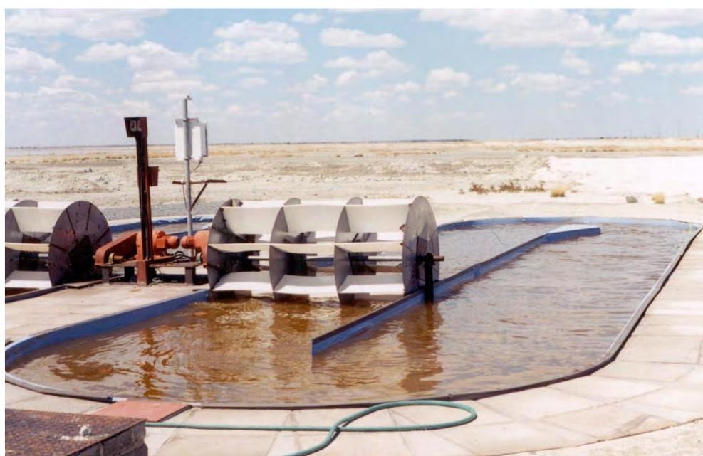
**Figure A5:** The *Dunaliella*-HRAP pilot plant treating saline carbonate brines at Botswana Ash Co. Sua Pan, Botswana
