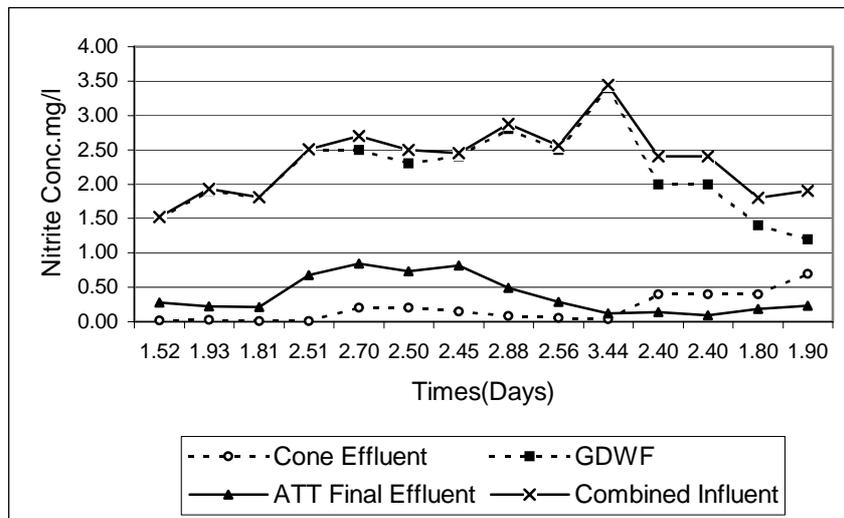
**Figure 9.8:** Nitrite removal in the algal denitrification packed column reactor showing influent nitrate and algal load drawn from the I-HRAP and set at a hydraulic retention time of 48 hours.
