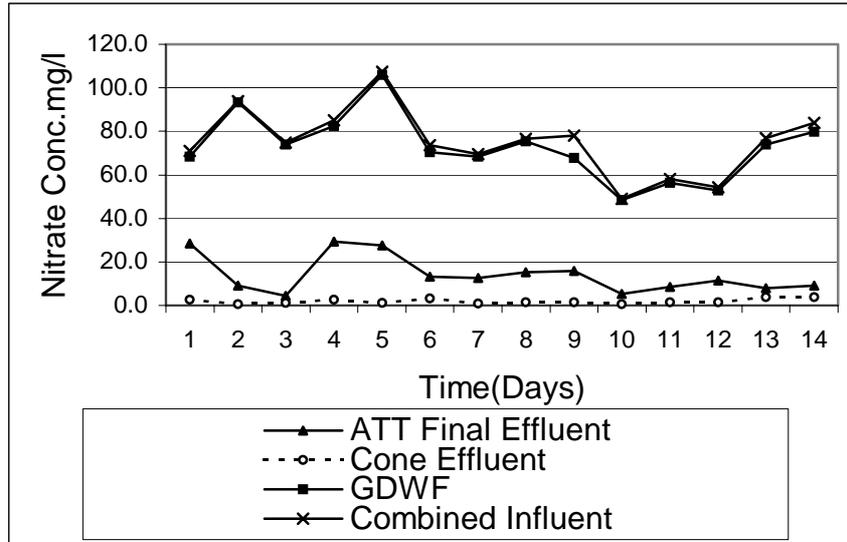
**Figure 9.7:** Nitrate removal in the algal denitrification packed column reactor showing effluent nitrate and algal load drawn from the I-HRAP and set at a hydraulic retention time of 48 hours.
