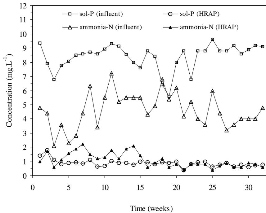
**Figure 7.2.** Treatment of GDW-final water in the I-HRAP over a 32-week period, indicating the phosphate removal effect.
