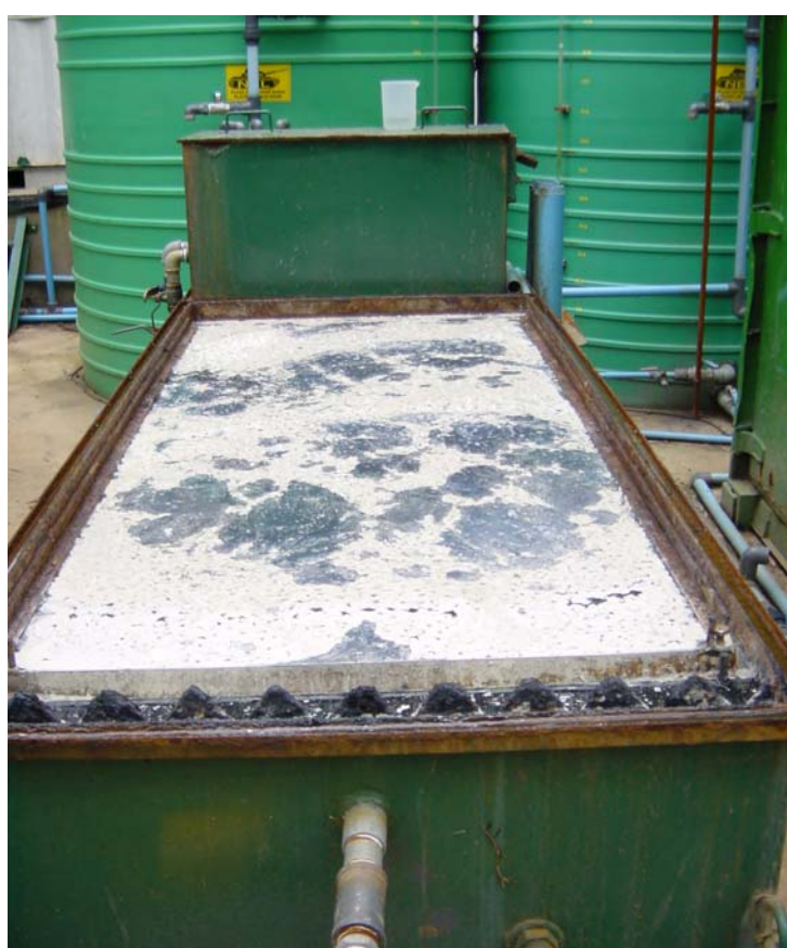
Figure A3.3. Bacterial extracellular sulphur catalyses the formation of polysulphide in the presence of sulphide at redox values around -150 \text{ mV} . At the air/water interface this is followed by the crystallisation of ortho-rhombic sulphur.
