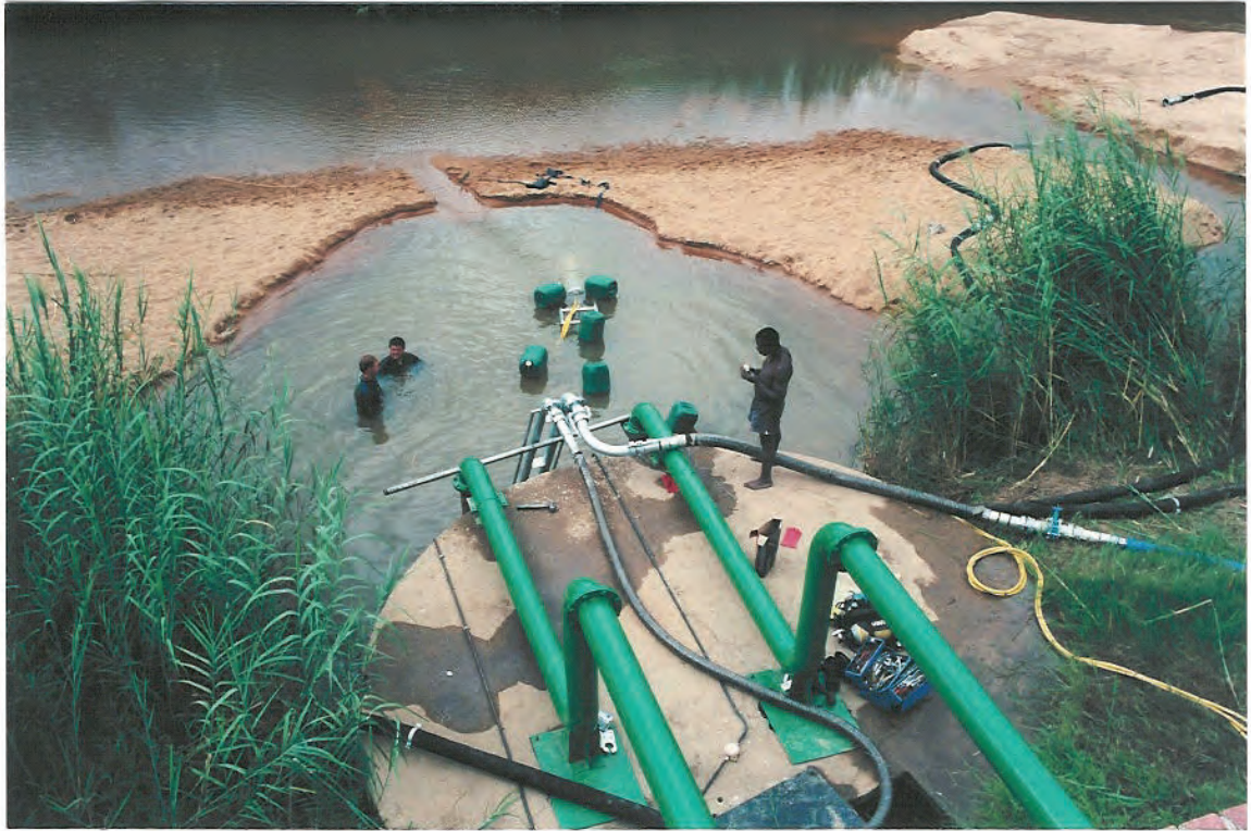
Figure 6-30 Mobile jet pump system mounted on trailer in operation (Bosman et al, 2003)
