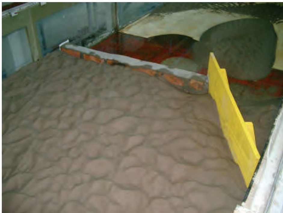
Figure 11-41 Bed forms after test run
