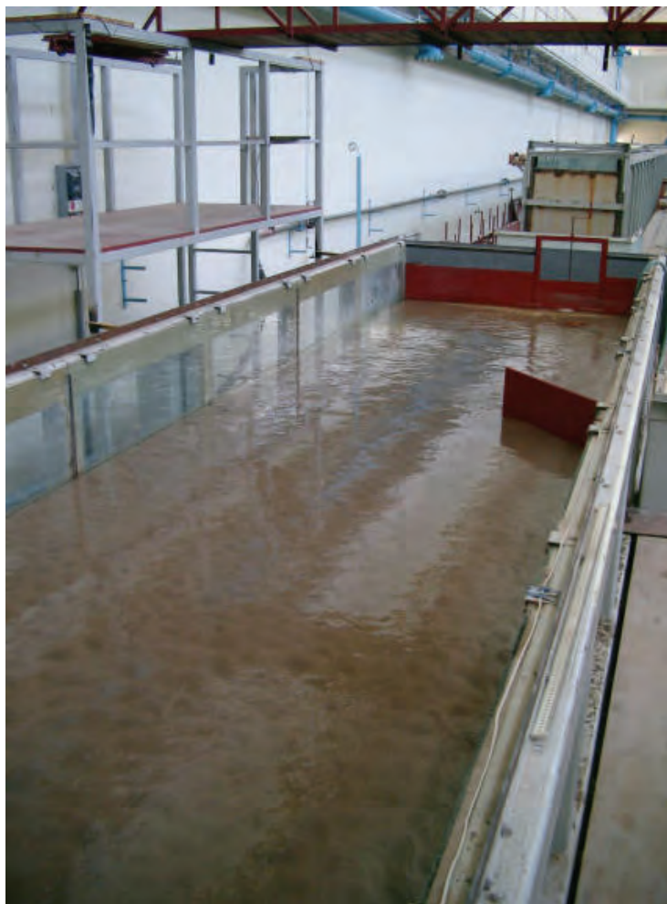
Figure 11-23 45 degree groyne with level water
