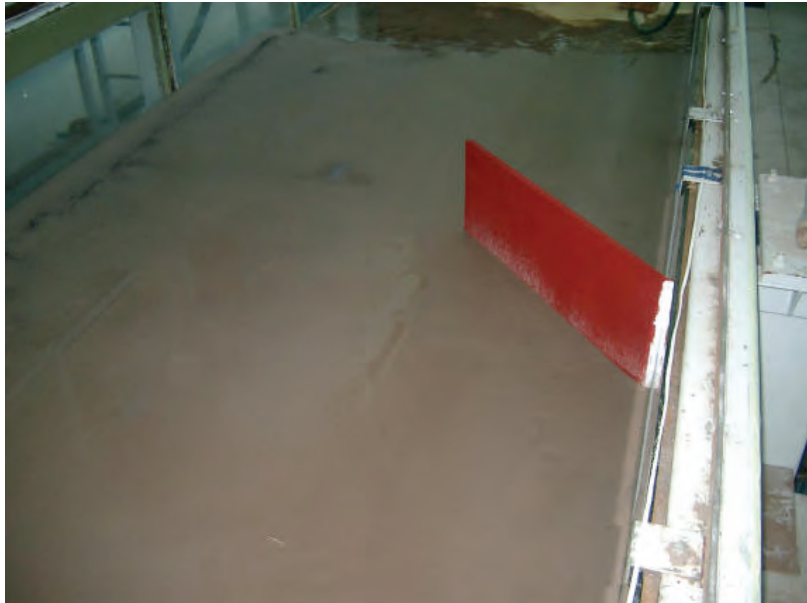
Figure 11-22 45 degree groyne with level sand before test
