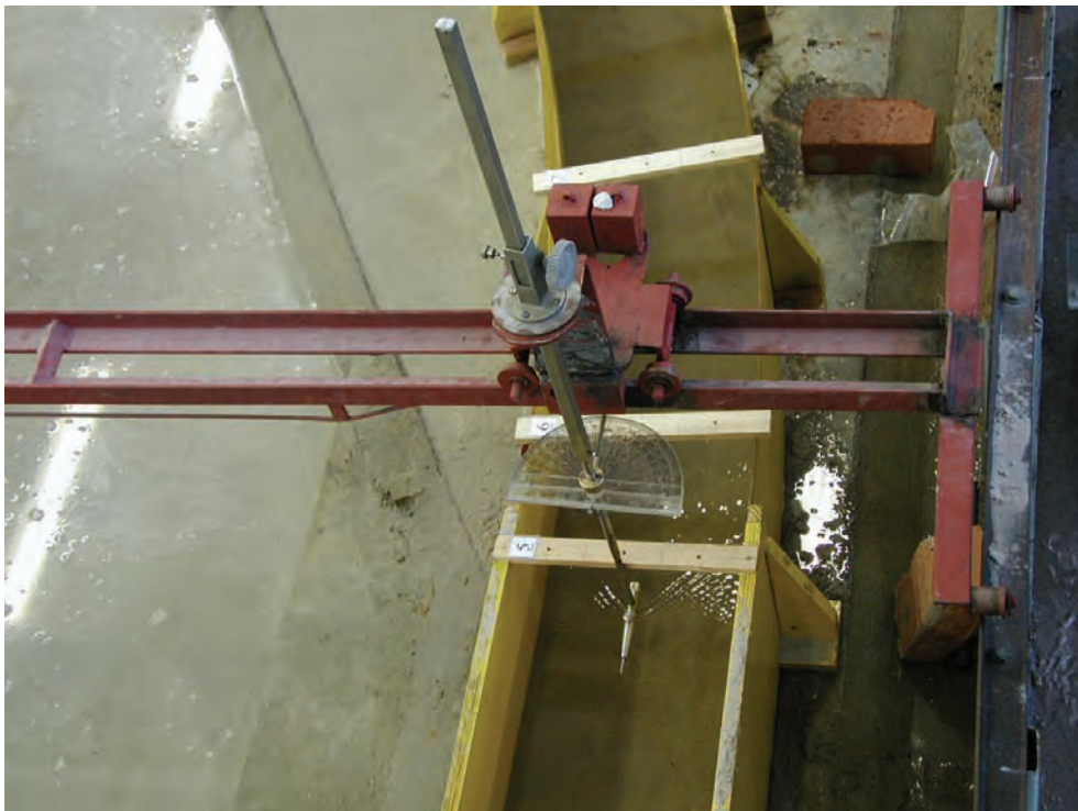
Figure 9-6 Velocity measurements with an A.Ott-meter
