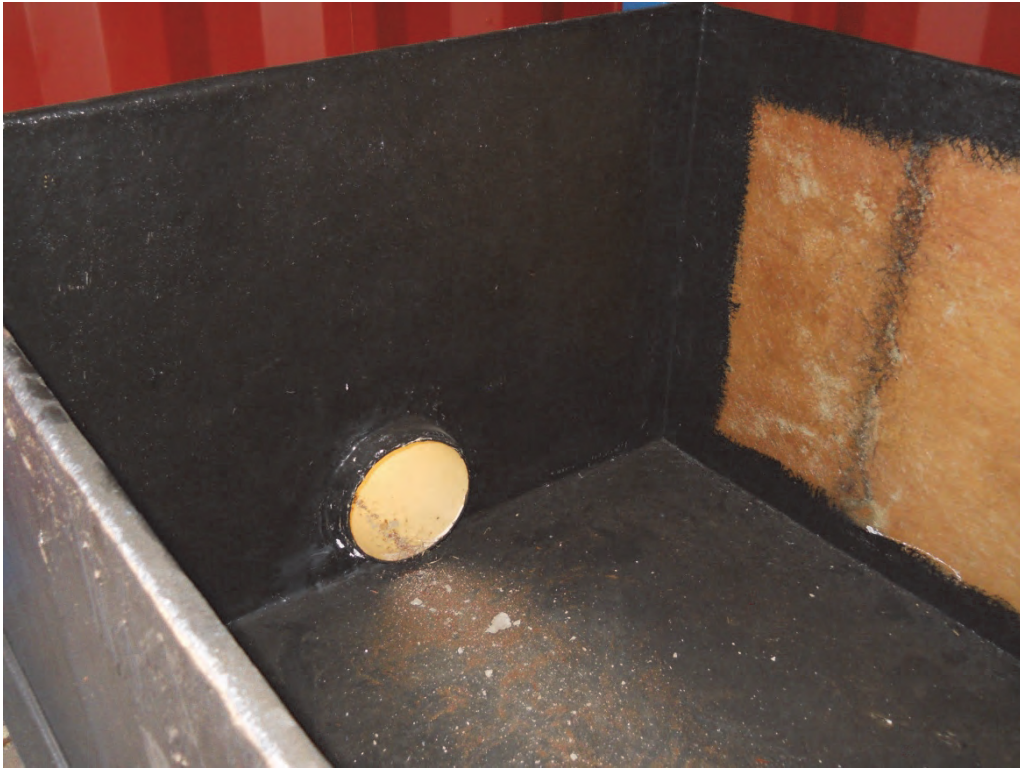
Figure 5-20: Collection box (underneath turbines)
