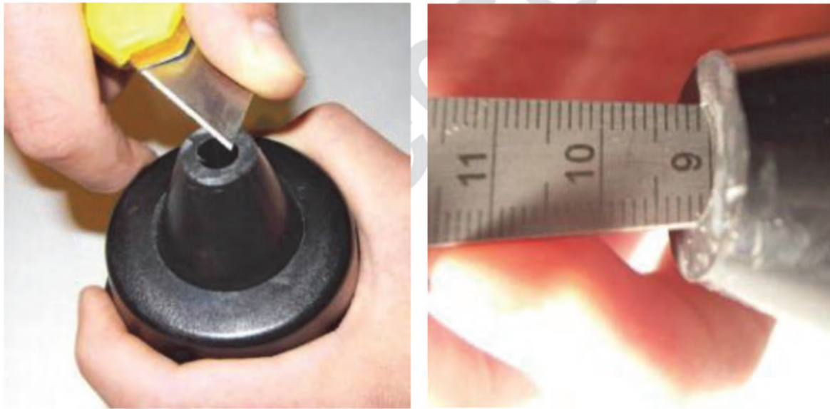
Figure 5-23: Cutting the jet to size and checking it with the taper gauge
