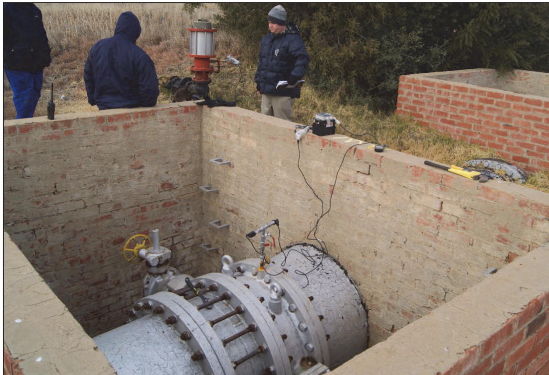
Figure 4-19: Setup of the pressure transducers at UB7 and UB8 (at Brandkop Reservoir)
