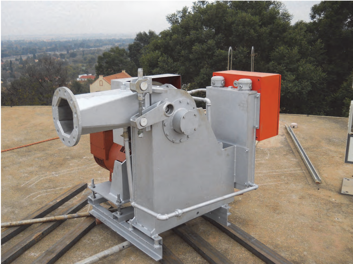
Figure 3-62: Crossflow turbine hoisted onto the reservoir roof
