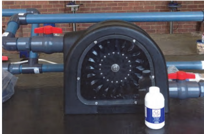
Figure 5-31: Ball valves and PVC manifold
