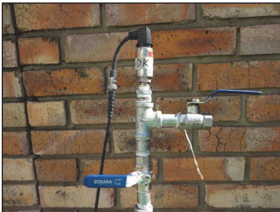
Figure 3-9: Pressure transducer with T-piece connector to expel air
