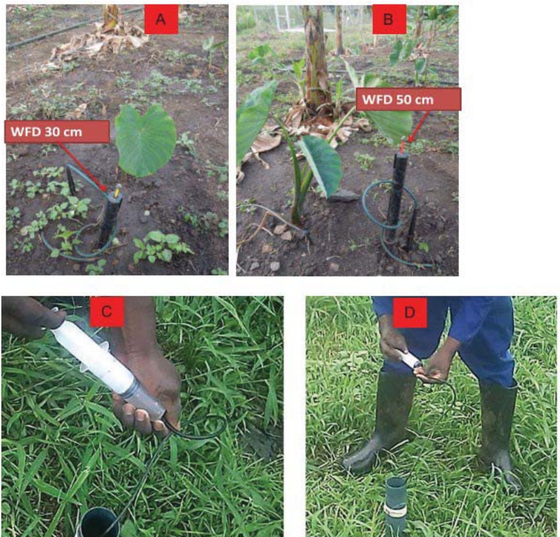
Figure 2.9: Toolkits for sampling leachates using wetting front detectors (WFD) (A=300 mm and B=500 mm depth) and piezometers (C and D). Adapted from Odindo et al. (2016).
