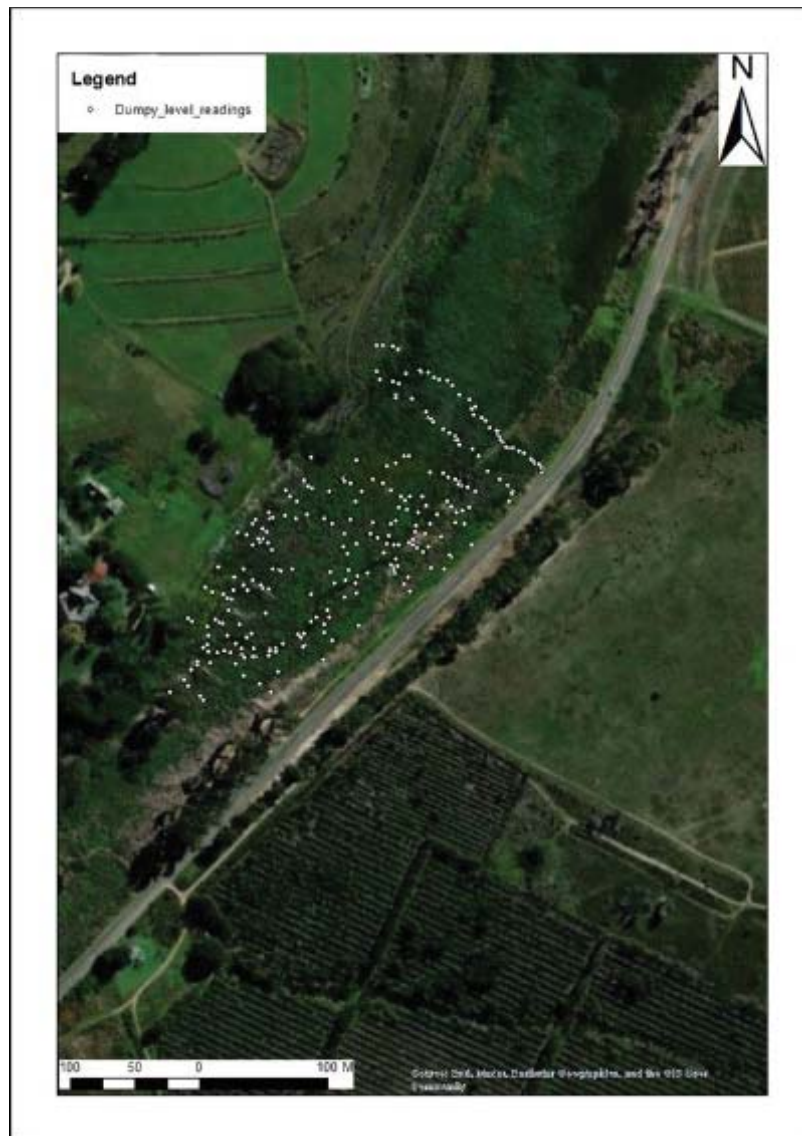
Figure 2.17 Surface elevation survey points along the Onrus Peatland, Western Cape.
