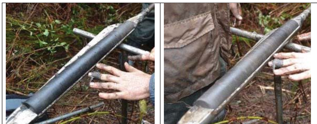
Figure 3.2 Spatial variation of peat/organic material. The peat/organic sediment layers were interrupted by mineral sediments (predominantly fine grained but with some sandy layers) suggesting a “punctuated/interrupted” aggradation of the peat/organic sediments.
