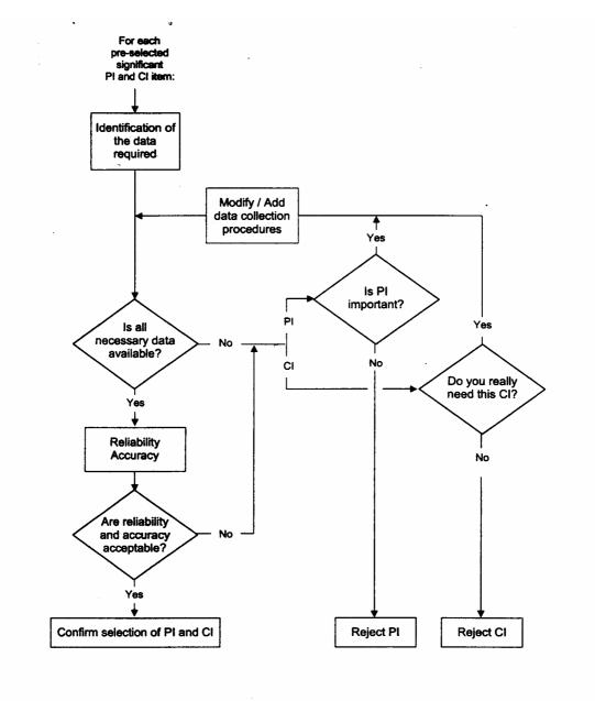
Figure 8. Pl and Cl selection procedure.
