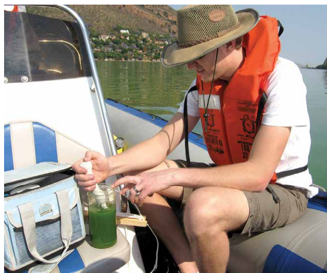
Dr Mark Matthews analyses a water sample during a field trip on the Hartbeespoort Dam in October 2010 to collect in situ bio-optical data, which he used during his PhD research to develop and validate the MPH algorithm.
