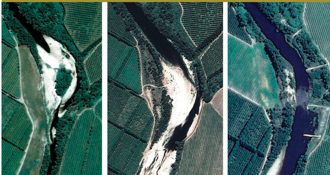
The progression of erosion on a bend in the Buffeljags River and subsequent recovery after groyne construction in 2012. From left to right: 2004, 2011 and 2016.
