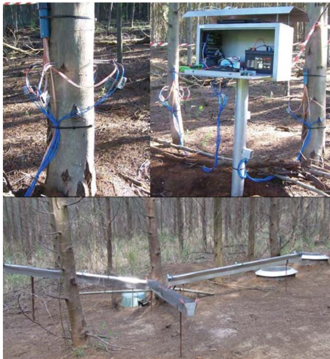
Figure 5. Monitoring of transpiration with the heat pulse velocity system and canopy interception at Two Streams research catchment.
