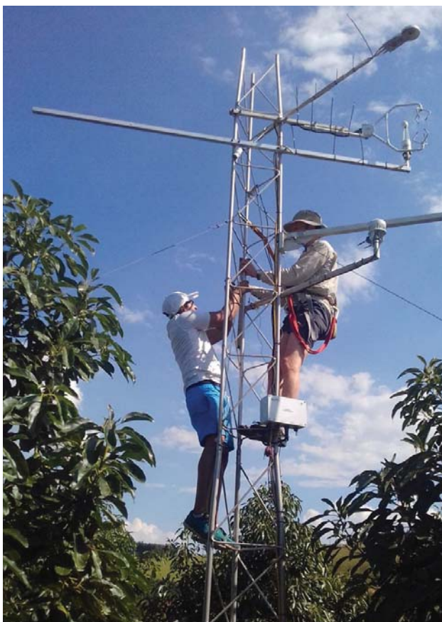
Researchers (left to right) Ruvekh Singh and Alistair Clulow rig up an eddy covariance systems at the intermediate orchard in Howick.
