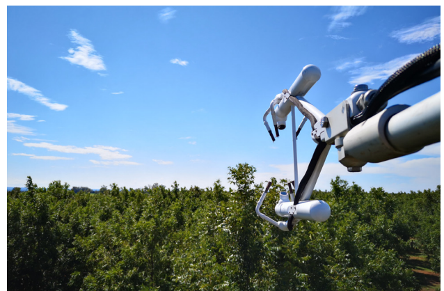
The infrared gas analyser and 3D sonic anemometer which forms part of an eddy covariance system. These instruments aid in the determination of water vapour and CO 2 fluxes, which when combined with other measurements can be used to estimate evapotranspiration.
