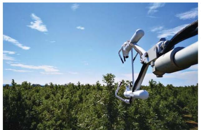
*The infrared gas analyser and 3D sonic anemometer which forms part of an eddy covariance system. These instruments aid in the determination of water vapour and CO<sub>2</sub> fluxes, which when combined with other measurements can be used to estimate evapotranspiration.*
