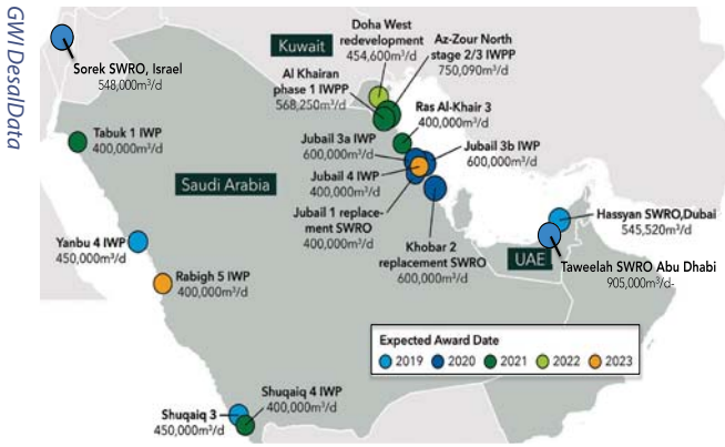
Figure 1: Fifteen mega-projects (>300MI/d) installing SWRO technology in the GCC region during 2019-23.
