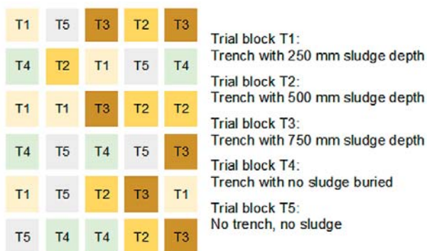
The layout of the 30 treatment blocks at the study site. Six trenches oriented downslope were dug in each of the 20 m x 20 m blocks.
