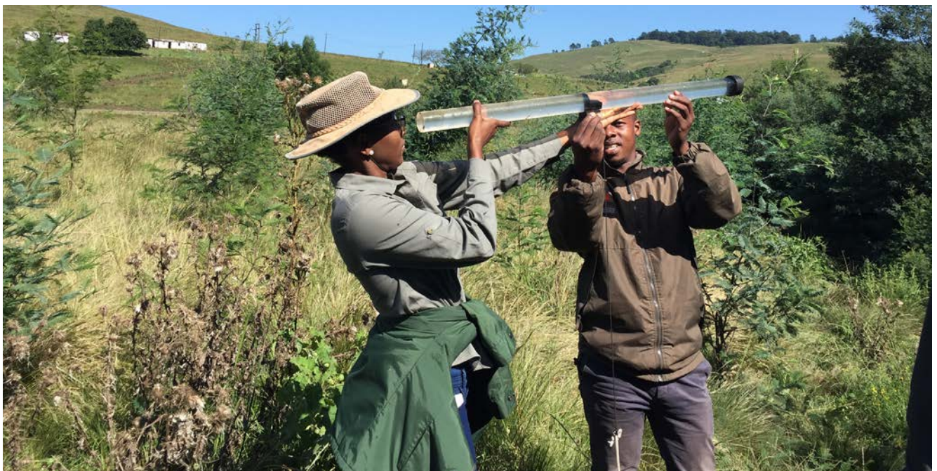
A clarity tube, used to measure water turbidity and suspended solids.
