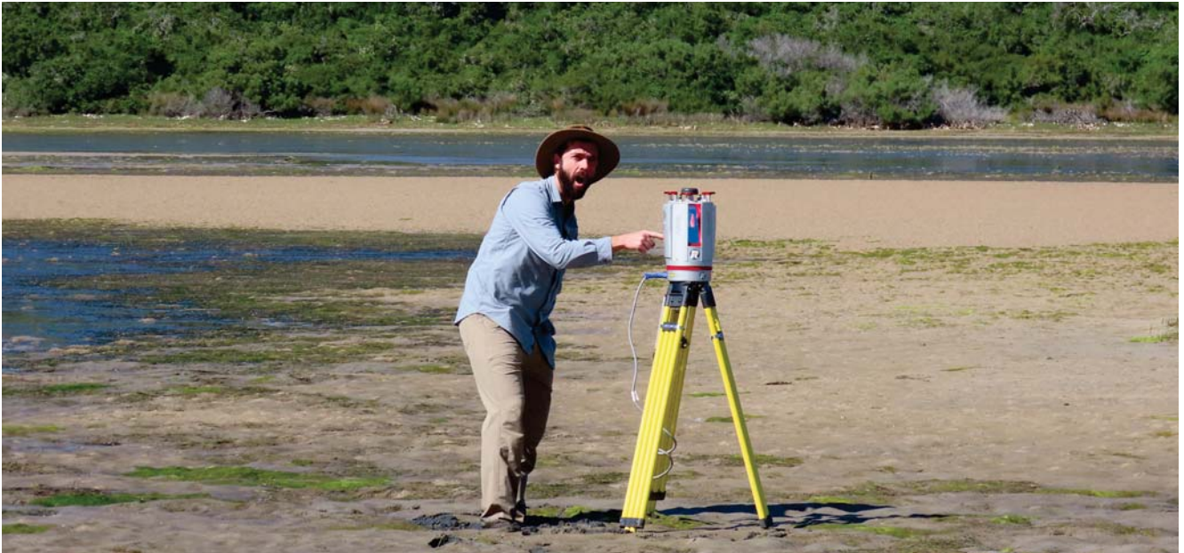
Figure 9: Dr Atticus Stovall collecting 3D data with a terrestrial laser scanner for mapping wetland topography and vegetation structure in the tidal estuary ecosystem.
