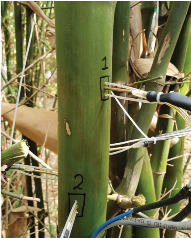
A bamboo stem at Shooter's Hill farm with probes inserted to measure sap flow using the heat pulse velocity technique.
