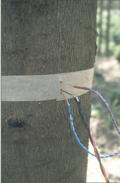
The heat pulse technique was used to measure the flow of sap in the sapwood of the tree
