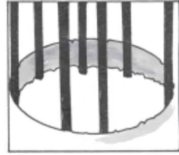
Plant the side poles or droppers firmly into the bottom.
