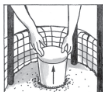
Pull the bucket partially out, leaving the stones in position. Fill the bucket again with stones and backfill with soil. Repeat for each layer.
