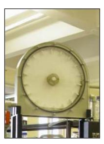
At the centre of the Rotoscope is a rotating plastic wheel that is half submerged in the main process water. Biofilm forms on the disc and is measured by green and/or infrared light that is projected onto the back of the disc (which is covered). The front of the disc is clear, which means the system could also be used to visually monitor algal growth, where relevant.
