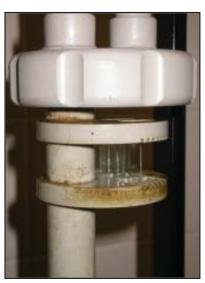
Inside this section of pipe is a series of removable glass slides. Biofilm forms on these slides as well as the plastic wheel, and while the wheel provides for real time monitoring, the slides give the user the option of sending samples away for more in-depth analysis and testing, if required.
