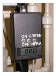
A digital measuring unit is linked to the red/green light box on the back of the plastic wheel. This unit measures the refraction of the light, which changes as biofilm forms on the wheel's white surface. When a pre-determined threshold is reached, the unit send a signal to the chemical dosing unit and a slug dose is released into the main water tank of the system.
