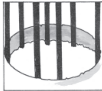
Plant the side poles or droppers firmly into the bottom.
