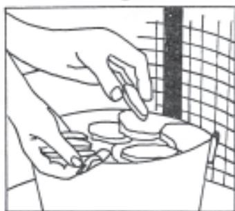
Pack stones carefully in the bucket to make sure that the water does not run through too fast.
