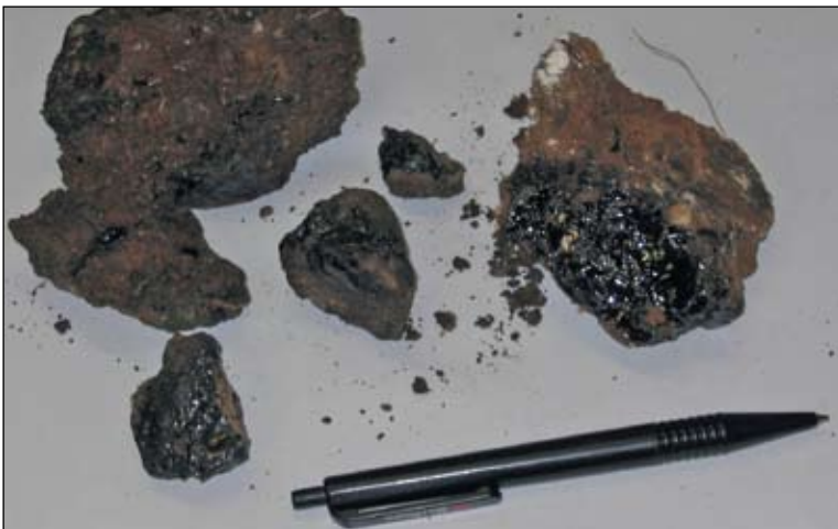
DNAPLs trapped in the subsurface act as continuing sources of dissolved contaminants to groundwater.
