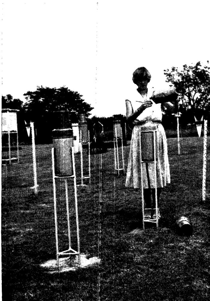
Figure 1 Rainfall from a standard raingauge being measured. Standard and plastic raingauges randomly arranged in 1,5 m x 3 m x 5 raingauges/row
