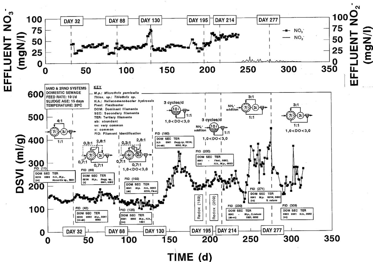
Figure 7 Sludge settleability as DSVI (ml/g), effluent nitrate ( $\text{NO}_3^-$ ) and nitrite ( $\text{NO}_2^-$ ), and changes in system operation with time (d) for System 5 in which the effect of differences between IAND and 2RND configurations were examined
