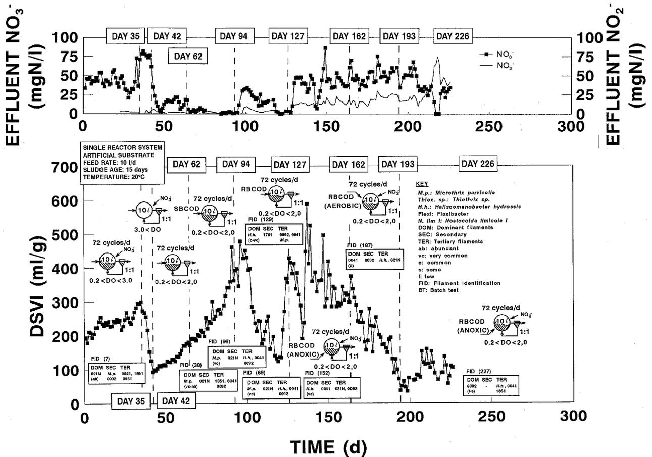
Figure 4 Sludge settleability as DSVI (ml/g), effluent nitrate (NO<sub>3</sub><sup>-</sup>) and nitrite (NO<sub>2</sub><sup>-</sup>) concentrations and changes in system operation with time (d) for System 2
