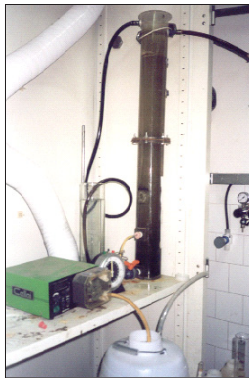
Figure 2 UASB pilot plant
