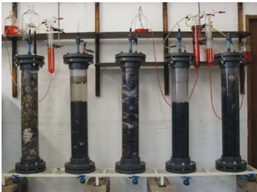
Figure 5 From left to right: Column 1: untreated waste; Column 2: under-sieved treated for 16 weeks; Column 3: over-sieved treated for 16 weeks; Column 4: under-sieved treated for 8 weeks; Column 5: over-sieved treated for 8 weeks
