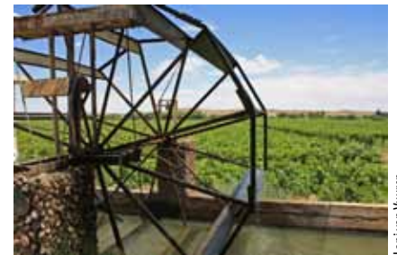
One of the most famous water wheels in South Africa is situated at Keimoes in the Northern Cape. The design is based on the Noria water wheel created in the Middle East during ancient times.
