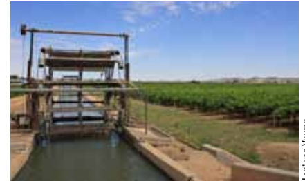
For many years the faithful water wheels at Kakamas have been used to move water from one irrigation canal to another.
