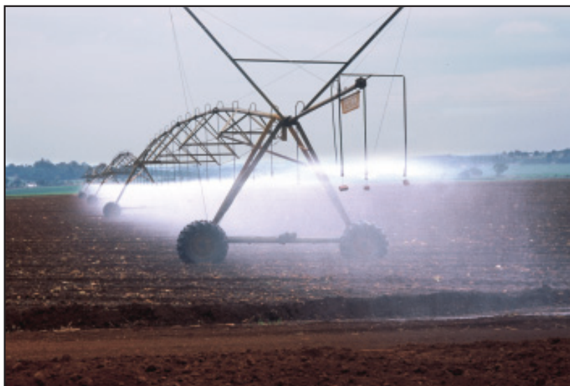
The modern centre pivot creates a microclimate and manageable infiltration rates
