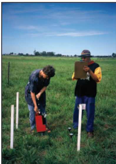
Astrid Hattingh (soil scientist) and Dalyn Ludick (pasture technician) measuring soil water content on the calibration plot
