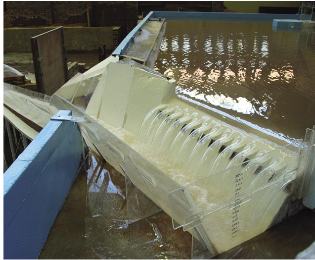
A scale model shows how the Berg River Dam will be prevented from overflowing. Excess water will spill over a 40 m spillway and flow down a deep concrete chute to a ‘ski jump.’ After being thrown 30 m up into the air, the water will land in a plunge pool 80 m away.
