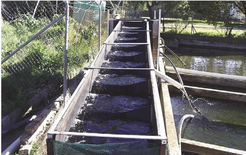
A close-up of an experimental sloping-baffle pool and weir fishway set up at the Dept. of Ichthyology and Fisheries Science at Rhodes University, Grahamstown.
