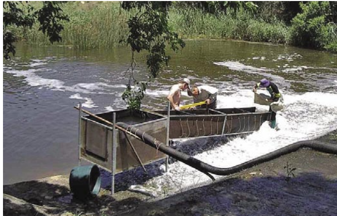
A portable experimental fishway being set up on the Kowie River ‘Ebb & Flow’ Weir.
