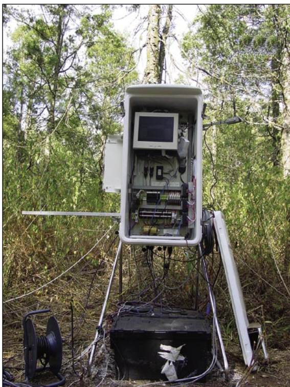
The surface layer scintillometer for the first time ever in South Africa installed above a complex vegetation type in South Africa: a Chromolaena odorata and Coastal bushveld/grassland mix in the Hluhluwe Nature Reserve.
