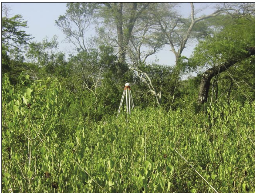
The surface layer scintillometer for the first time ever in South Africa installed above a complex vegetation type in South Africa: a Chromolaena odorata and Coastal bushveld/grassland mix in the Hluhluwe Nature Reserve.
