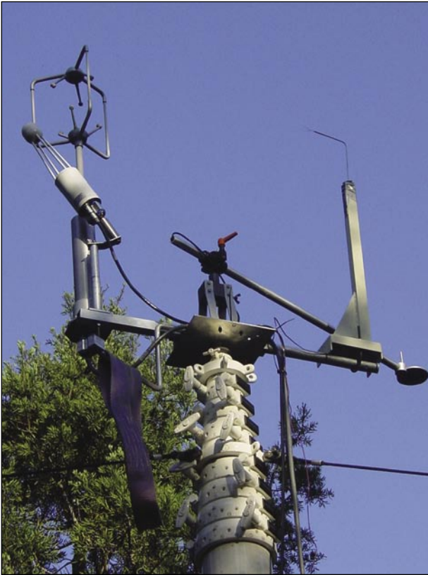
Gill Sonic anemometer and Li-Cor gas analyser (dominant white, left) as part of an eddy covariance system installed at the top of a telescopic mast at the Podocarpus falcatus research site in Tzaneen, in addition to the thermocouple and net irradiance sensors (right).
