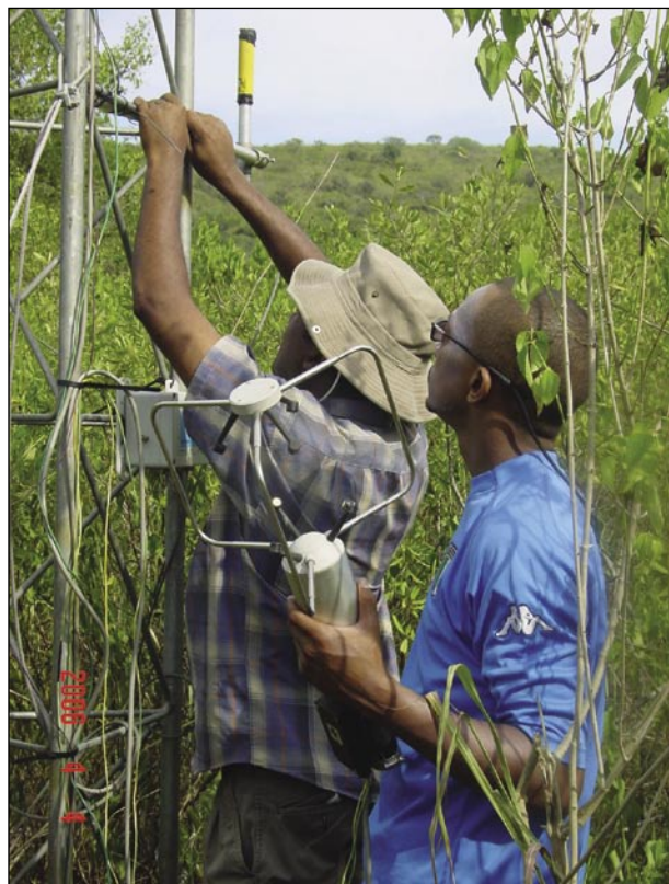
The large aperture scintillometer receiver sensor installed above a mixed stand of Chromolaena odorata and Coastal bushveld/grassland.
