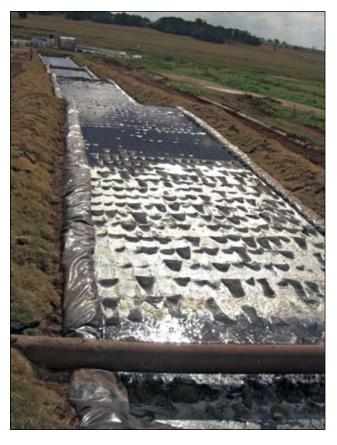
process. After a few days the mine-water is run through the different bags filled with bark and needles. The precipitation is then visible on top of the bags.
