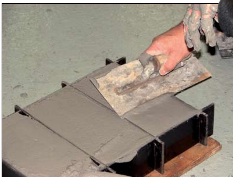
UP concrete technologist Derek Mostert demonstrates the ease of casting foam bricks.
