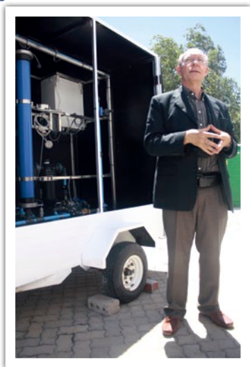
Ikusasa Water Marketing Manager Dr Gerhard Offringa explains the functioning of the firm's mobile water treatment unit. Units can produce between 200 and 400 l/h per module installed. A similar unit has been supplied to Cape Winelands municipality for use in emergencies.
