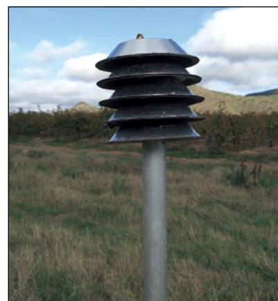
Loggers recording air temperature and relative humidity have been installed at some of the study sites to determine their relationship to water temperature.
