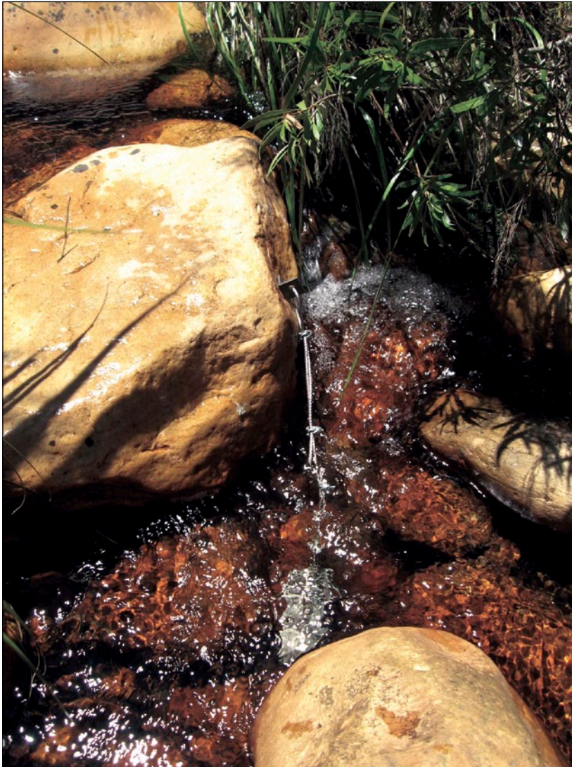
The water temperature loggers are housed in a protective metal casing and positioned in a run in the thalweg – the point of deepest flow.
