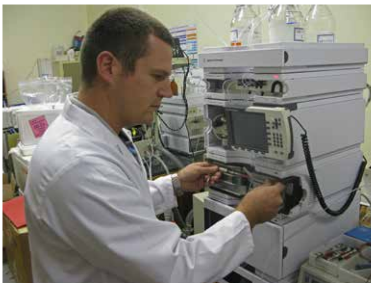
Christiaan Odendaal, a Ph.D. student in Environmental Management at the University of the Free State, attaches a column to a high performance liquid chromatography system which separates emerging contaminants before they are detected or quantitated in a mass spectrometer.
