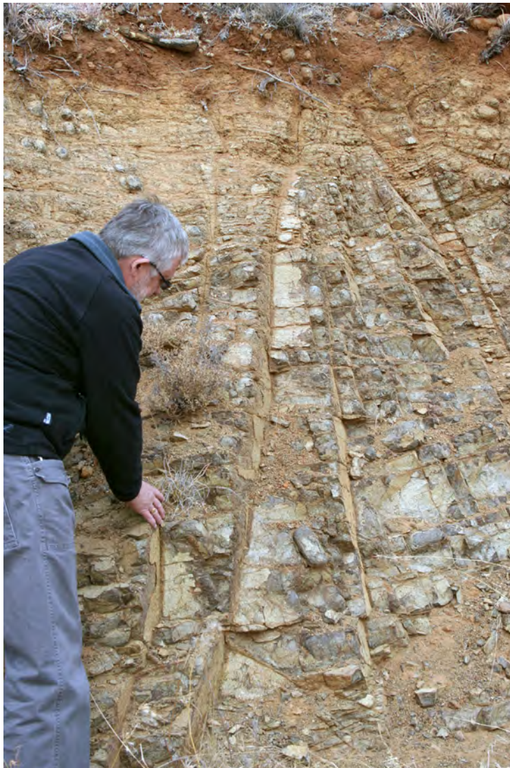
Right: Dr Eddy van Wyk of the Department of Water Affairs inspecting a dolerite dyke showing the fractured zones in the rock face at the western site.
