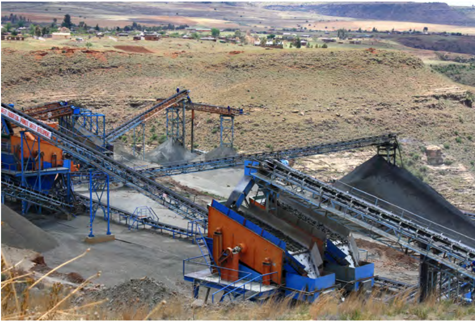
The aggregate processing system has a capacity of 400 t/h. On-site basalt rock is being used as concrete aggregate, while sand is crushed from the basalt stone due to the limited availability of natural sand sources.
